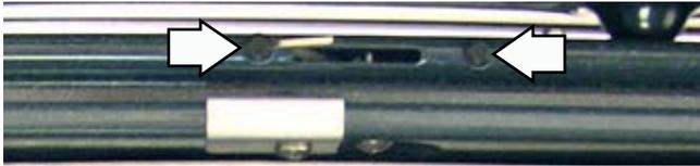
3. Disconnect the motor and switch wiring harnesses from the lock assembly.
