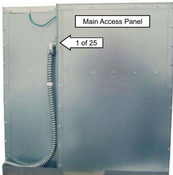
3. To remove the secondary rear access panel, remove the twenty-five 1/4-in. hex-head screws that hold the secondary rear panel in place.
