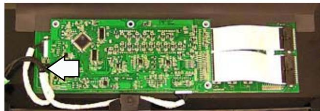
6. Disconnect the 2 ribbon cables from the right side of the board.
