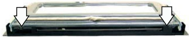
4. Remove the two T15 Torx screws (1 on each side) from the outer door assembly.
