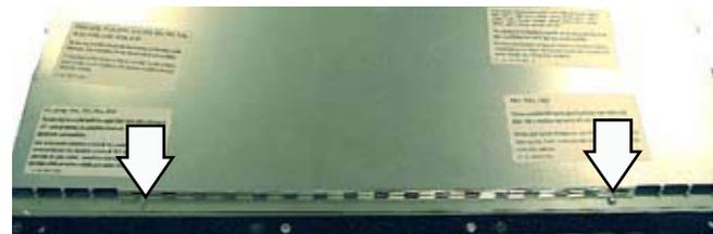
4. Remove the fifteen 1/4-in. hex-head screws from the sides and back of the oven that hold the top access panel in place. There are 4 screws on the left side, 3 screws on the right side and 8 screws on the back of the oven.
