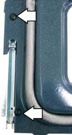
3. Remove the six 1/4-in. hex-head screws that hold the insulation retainer to the inner door. Remove the insulation retainer.
