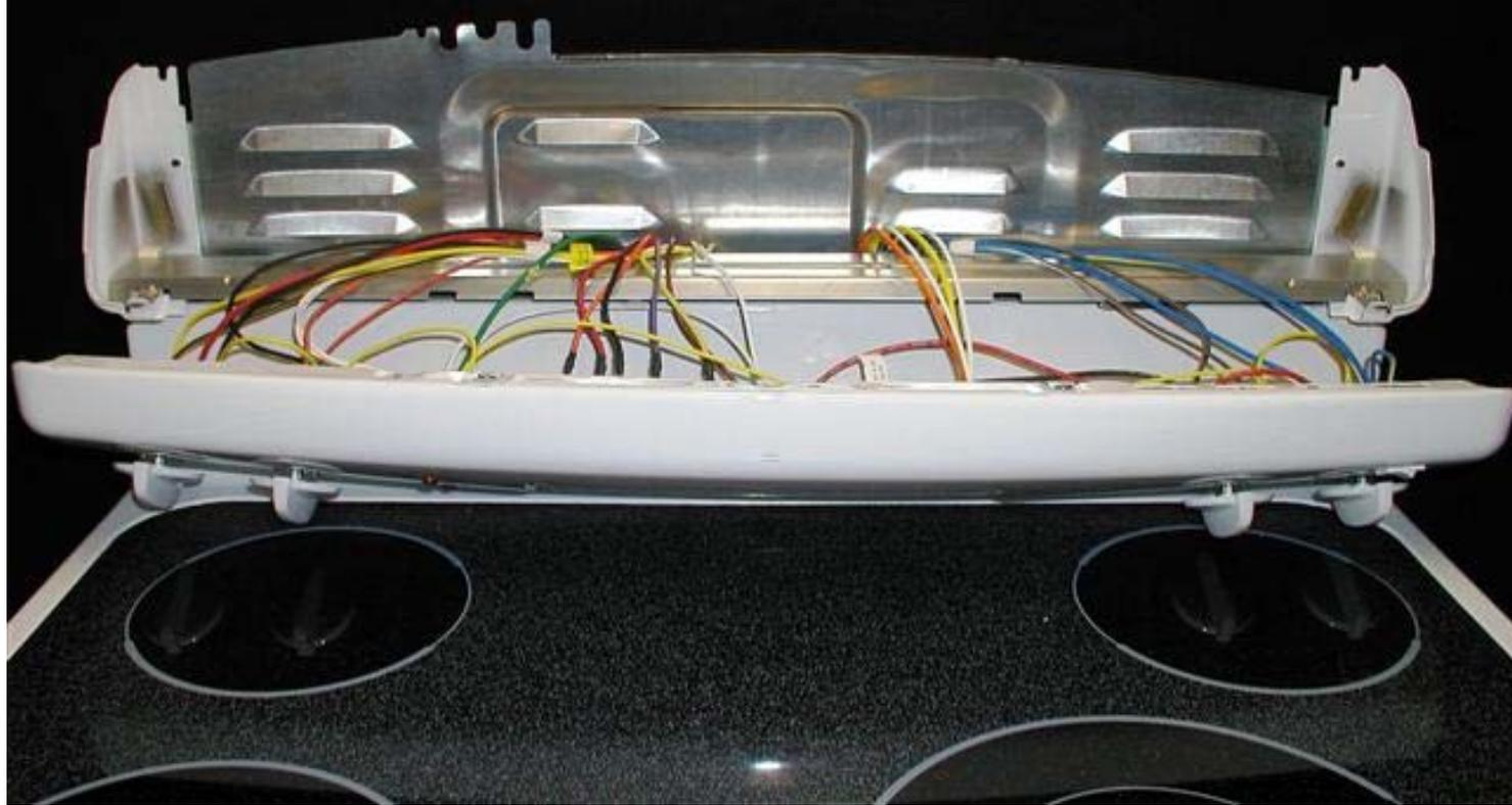
3. Pull bottom of panel out while lifting panel up.
