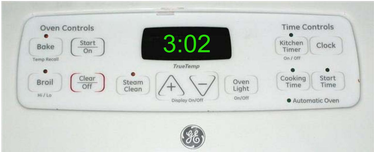
**Note:** the clock display will go blank if the UP and DOWN arrows are pressed at the same time for 1 sec or less.
