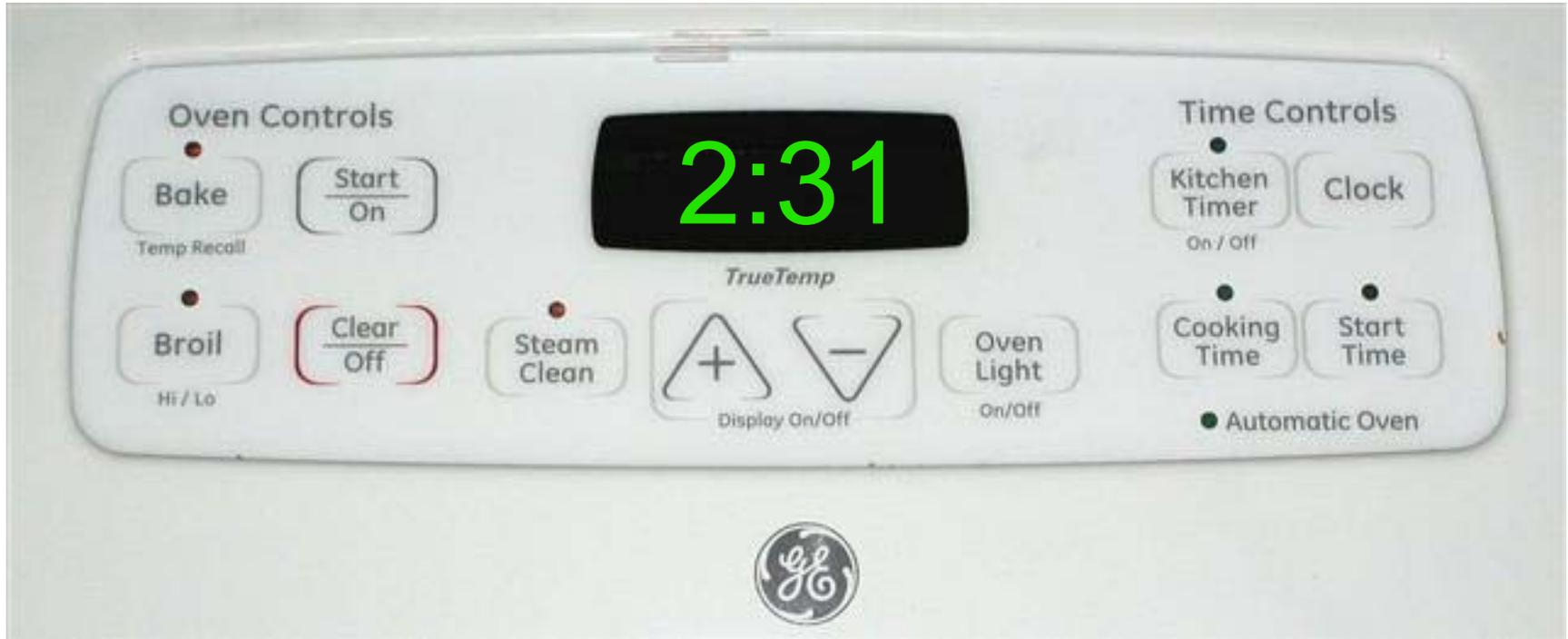
The T09 Control System consists of the control, the key panel and the oven sensor. (Control & key panel are a single component).
