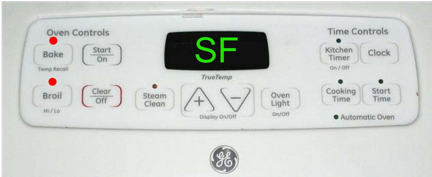
Hold **Bake** and **Broil** keys simultaneously for 2 seconds until display shows SF (Special Function). Select the area to change. When change has been made, press start key to return to time of day.
