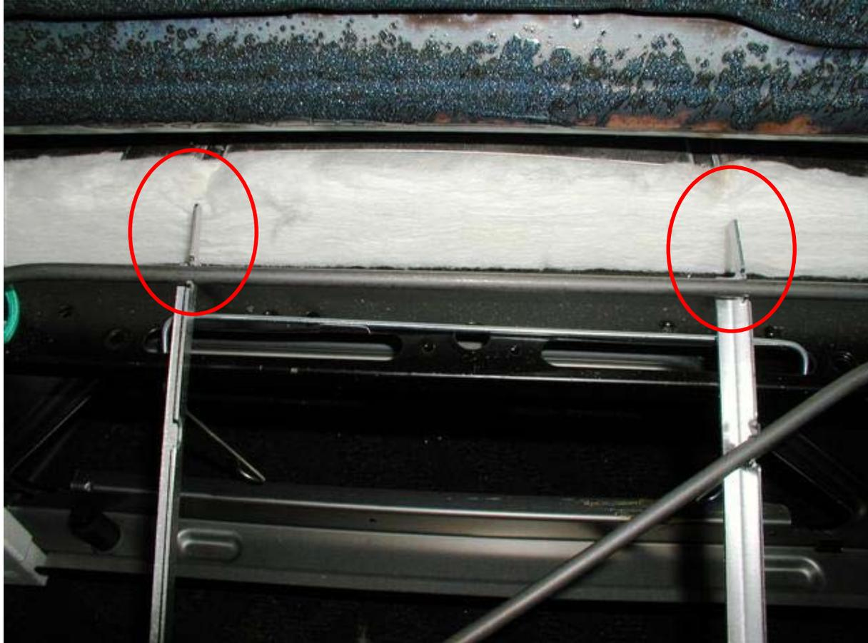
Upon re-insertion of bake element, tabs on assembly must align with slots or openings on the far side of the compartment.
