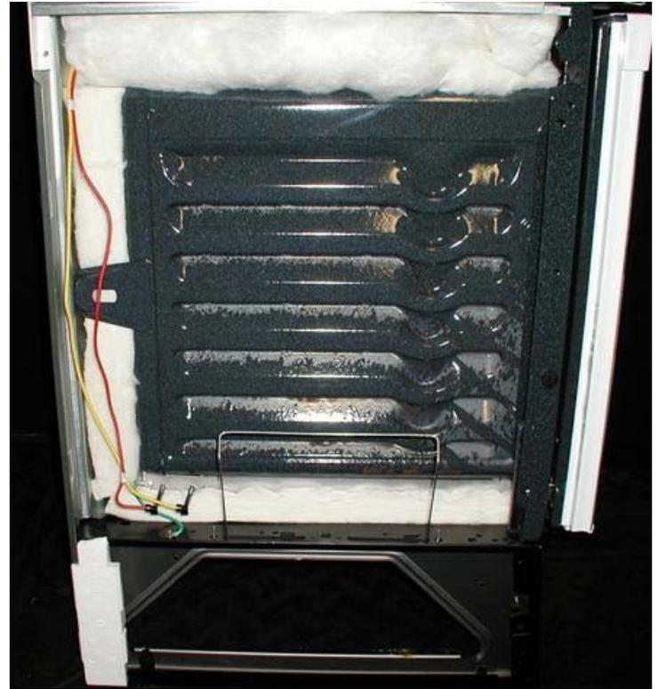
Carefully, lift insulation blanket and temporarily tuck it under upper frame to clear work area.
