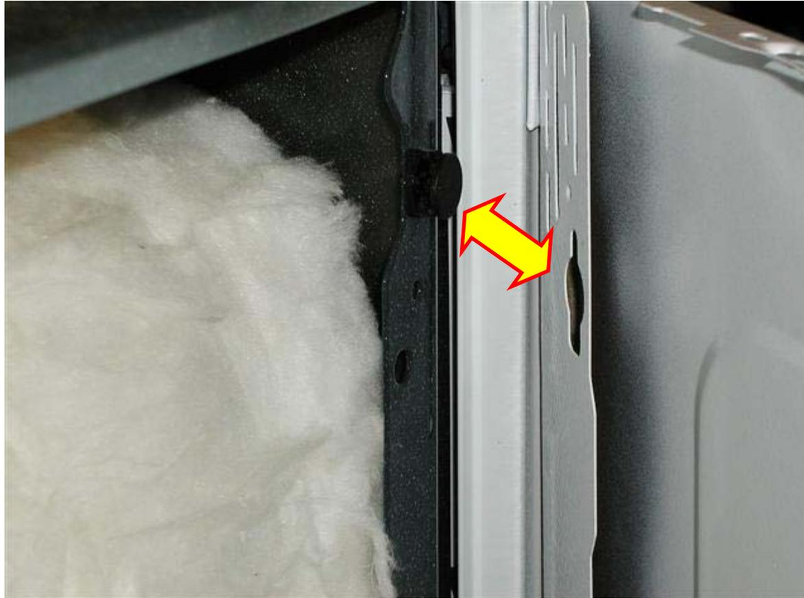
Finally, grasp panel and lift @ an inch to release tabs on the side of the frame from openings in the side panel.
