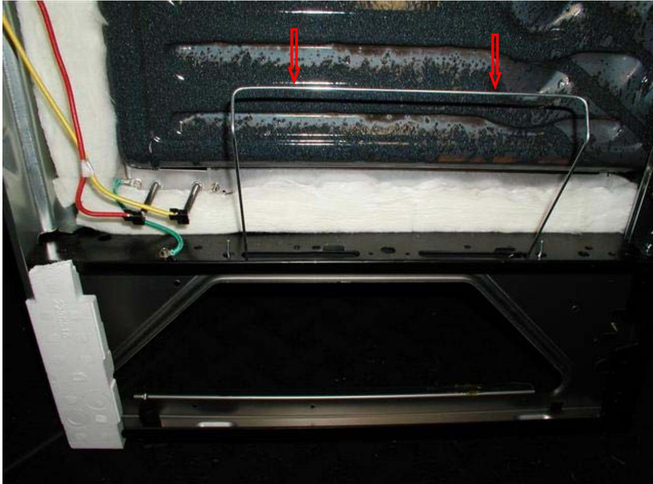
Push down on insulation retainer to clear it from the bake element compartment opening.
