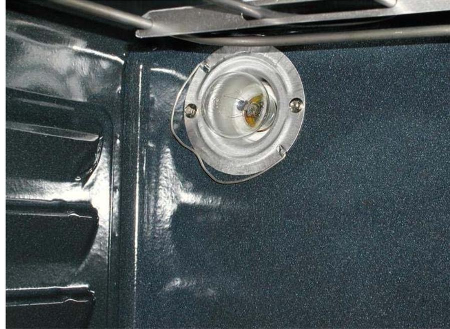
Oven lighting consists of a single 40w, incandescent bulb with a clear glass cover held in place with a spring wire.
