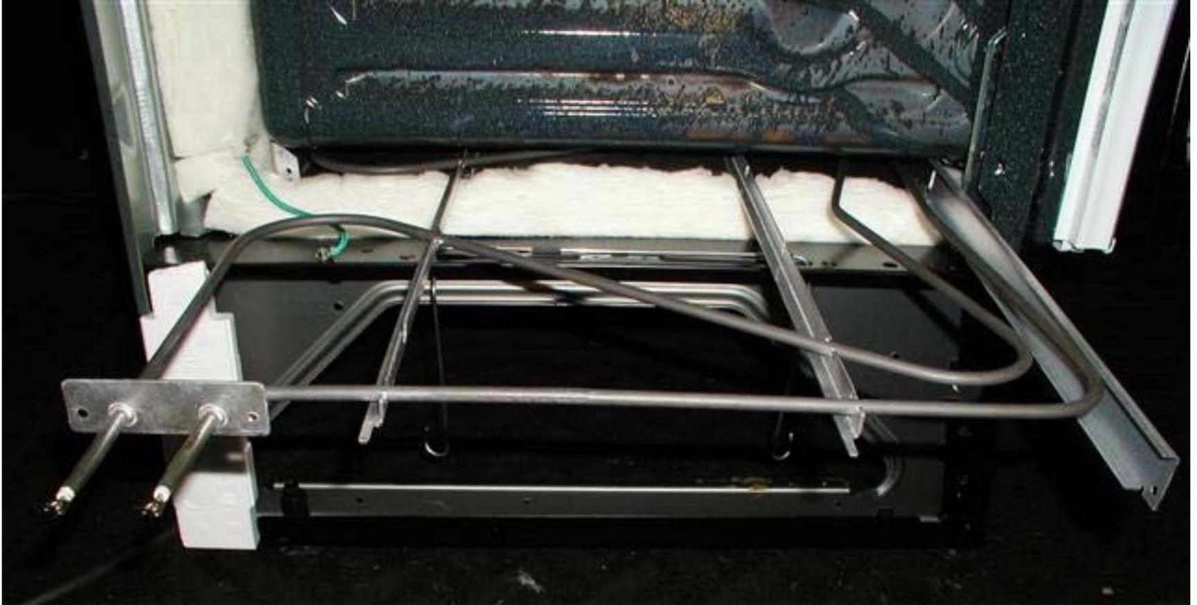
Slide out element from compartment to remove.
