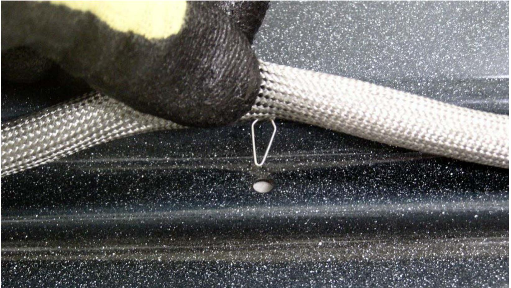
Door gasket attached with spring clips around perimeter of door.
