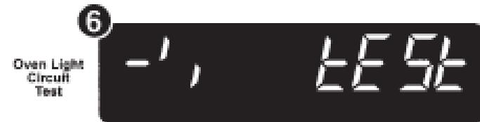
**7. ENERGIZE TOP PANEL LIGHT CIRCUIT** - To perform this test, press the TOP LIGHT key pad, and watch the top fluorescent light energize. As soon as you release the TOP LIGHT pad the fluorescent light will deenergize. If the light does not energize, check the following: reconfirm that you have entered the test mode correctly, check power and wiring connections to the ERC, check for a defective bulb, starter or ballast and lastly suspect a faulty ERC.
