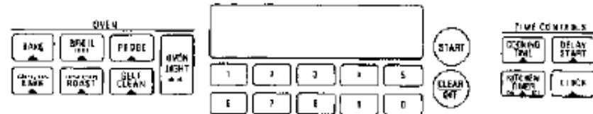
**Group 3 (ERCIII D) - Lower oven self clean control for double oven microwave built-in. Some models come with probe and convection feature.**
