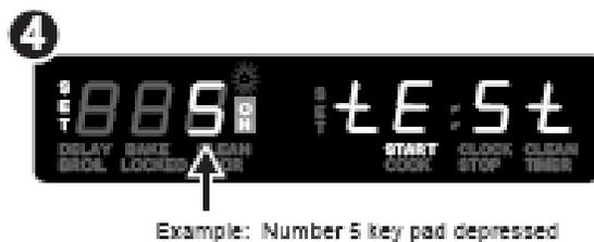
**4 NUMERIC KEY PADS TEST** - To perform proper numeric key panel input responses, press any numbered key pad and hold it in for approximately 5 seconds; the number you are pressing will show in the ERC display. If it does not, reconfirm that you have entered the test mode correctly, check wiring connections to the ERC and keypanel, and lastly confirm shorted or open key pad by performing the Key Panel test on page 10.
