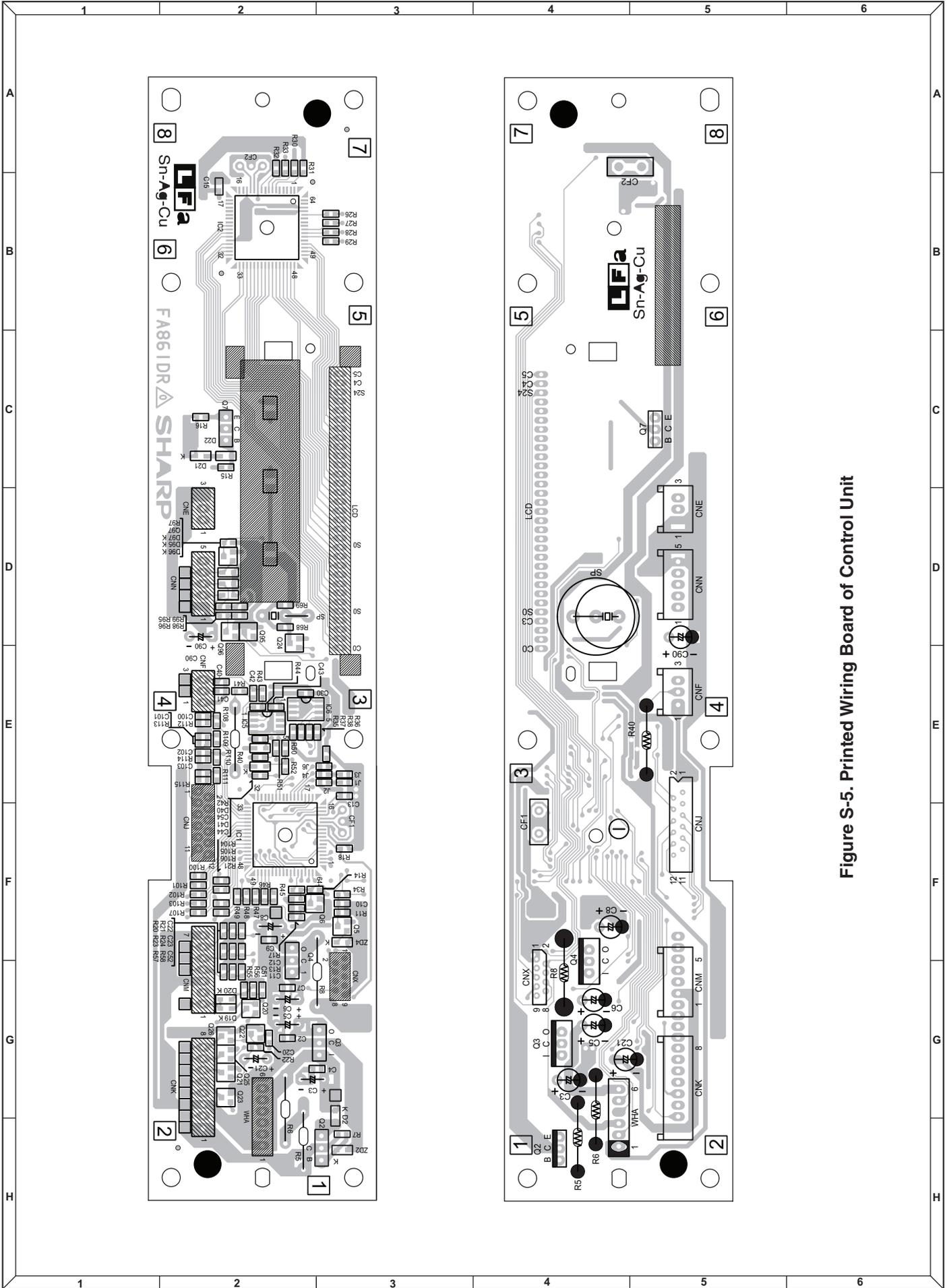
Figure S-5. Printed Wiring Board of Control Unit
