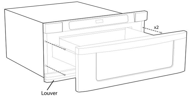
2. Open the Drawer to access the 4 mounting screws holding the unit on to the wall or cabinet opening. **(Fig 1)**.
