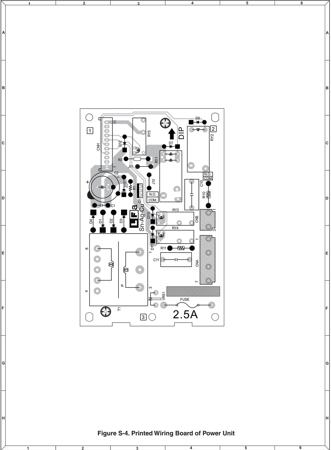
Figure S-4. Printed Wiring Board of Power Unit
