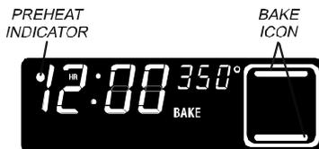
4. A single chime will indicate the oven is preheated to the set temperature. The preheat indicator will turn off.
