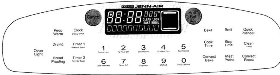
The electronic control is designed for ease in programming. The display window on the control shows time of day, timer and oven functions. Control panel shown includes Convect and other model specific features. (Styling may vary depending on model.)
