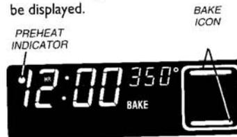
4. A single chime will indicate the oven is preheated to the set temperature. The preheat indicator will turn off.
