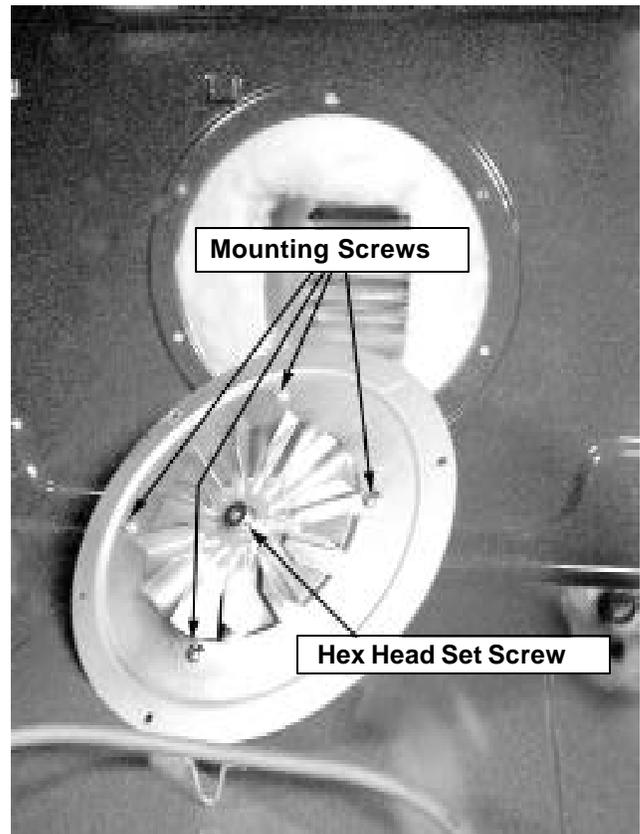
*Note: When reinstalling the convect assembly, be sure to check that no loose insulation is visible in the fan area or anywhere in the oven cavity.*
