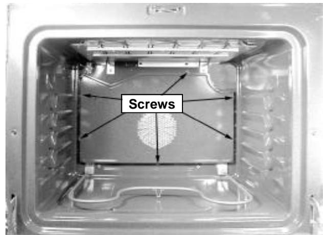
Three screws (shown) secure the convection fan mounting plate, remove these, to allow access to the motor and connectors.
