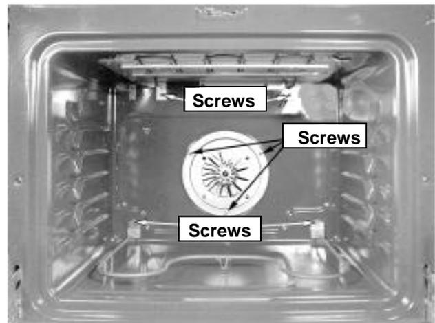
*Also shown here are the screws that secure the bake and broil elements.*
