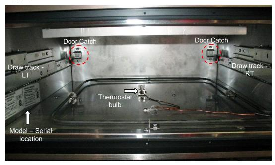
**Fig 10** shows a close-up of the thermostat cap tube routed through the hold down clamp and the senor bulb in its mounting bracket.
