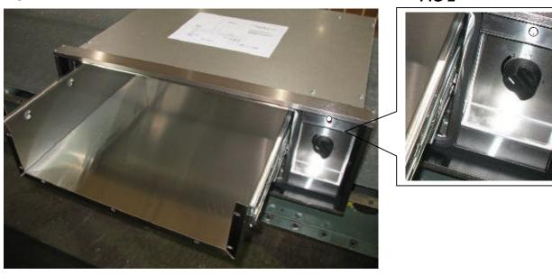
The temperature range of the warming drawer is between 90° F (Min) to 250"F (Max) The temperature is control by the thermostat. In order to gain access to the thermostat and power connections, removed the unit from the cabinet to expose the right side access panel. FIG 3 shows the cover installed (Outlined with dotted red line)
