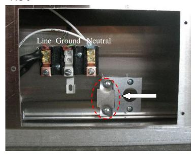
**FIG 6** shows the Component compartment where the thermostat control is housed. The Capillary tube of the thermostat is routed through the side wall to the sensor. In this same location is where the heating element connections are located. One side is wired directly to Neutral. The other to the Thermostat. The indicator lamp is directly above the thermostat (Not shown)
