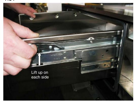
FIG 8 shows the draw being lifted away from the drawer tracks. Remove and place on a protected surface.
