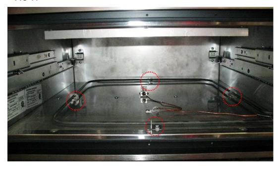
FIG 12 shows the right side entrance where the thermostat and heating element enter the chamber of the warming drawer. Remove the (2) screws shown to pull the heating element from the unit.
