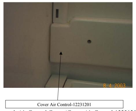
6) Reattach Air Control Cover (Cover-Air Control-12231201) to back of fresh food cabinet. Be sure to position Air Control Cover as far to the left as possible and tighten screws all the way so that gasket around perimeter of Air Control Cover compresses.
