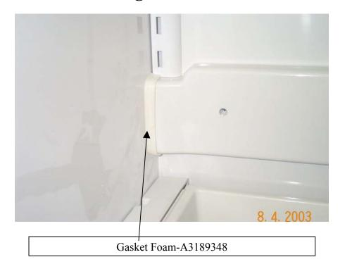
7) If air is still leaking or you see a gap on the left hand side of Air Control Cover, place Gasket Foam (Gasket Foam-A3189348) around the outside perimeter of Air Control Cover (Cover-Air Control-12231201
