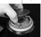
3. Use a T20 torx screwdriver and remove the two screws from each burner head, then lift the heads off the cooktop.
