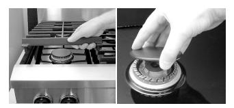
Use a 7 mm nut driver and remove the 6. orifices from each of the burners. NOTE: Place a small piece of masking tape along the inside edge of the nut driver to help keep the orifice in the driver.
