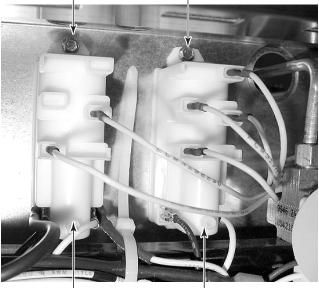
Spark Module For LF & RF Burners
