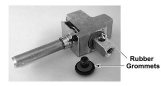
b) Remove the mounting screw from the gas manifold and remove the valve and its rubber grommet from the manifold.
