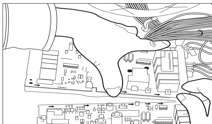
Figure 4-18. Light Transformer Removal.
