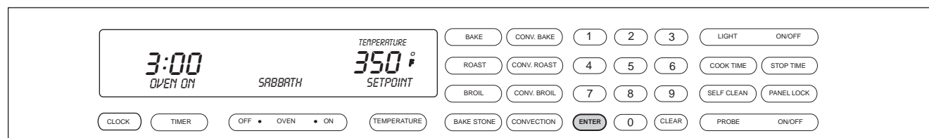
Figure 3-5. Now, press and HOLD THE ENTER key for 5 seconds. The oven will chime twice and the word Sabbath appears in the display.
