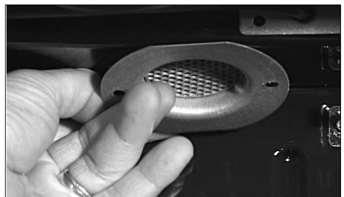
Figure 4-34. Smoke Catalyst Removal.
