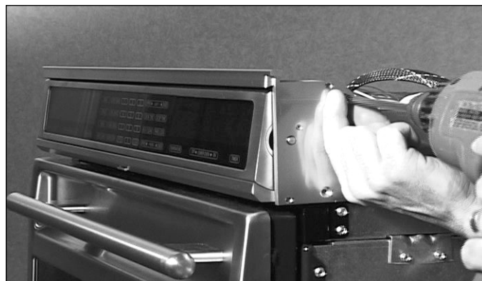
Figure 4-1. Control Panel Removal.
