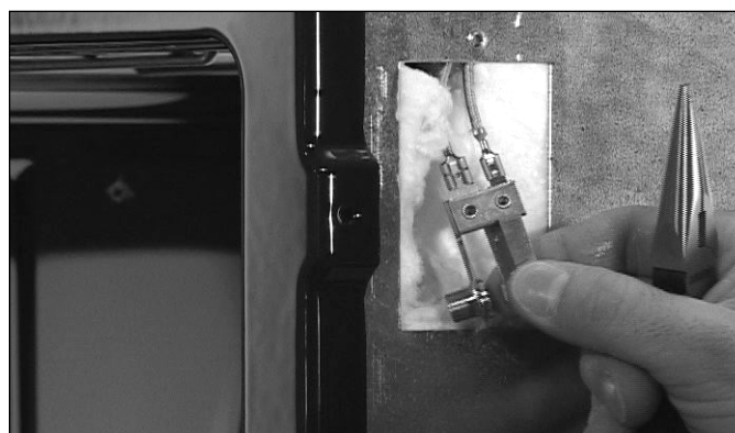
Figure 4-28. Probe Switch Removal.
