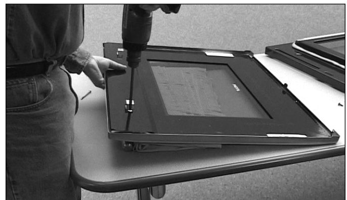
Figure 4-38. Outer Door Skin Removal.
