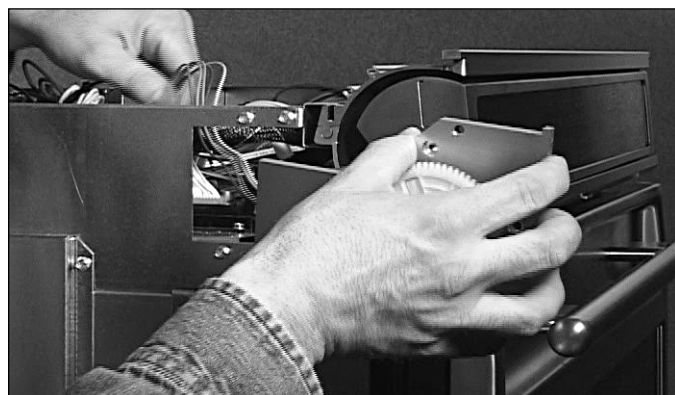
Figure 4-4. Control Panel Drive Motor Removal.
