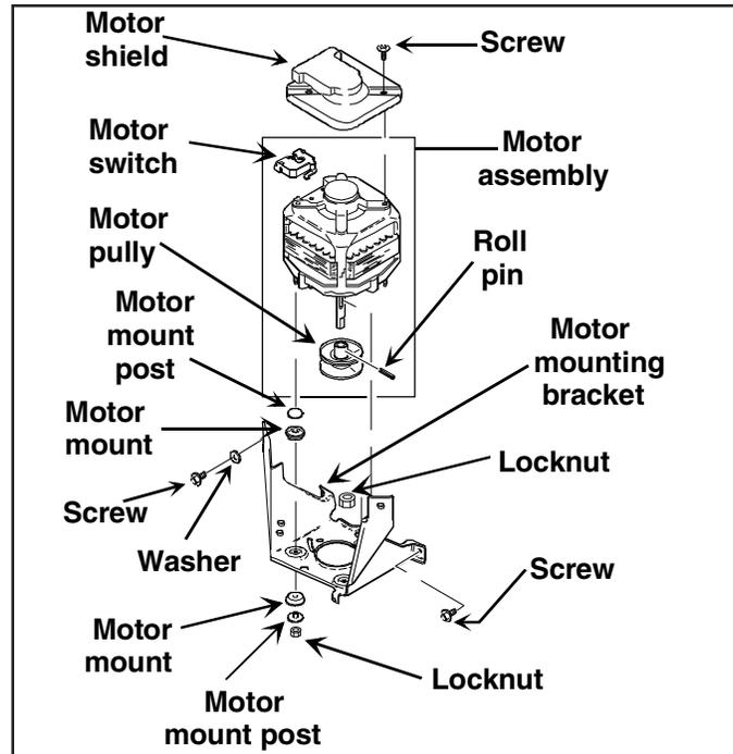
2. Lift motor off mounting bracket and remove remaining rubber mounts and steel washers from motor mounting studs.
