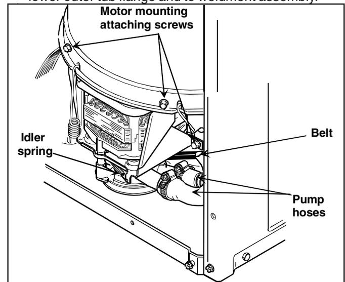
7. Lift complete assembly out of washer.
