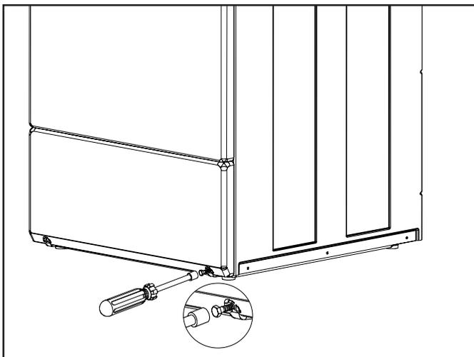
2. Remove lower screws in Front Panel.
