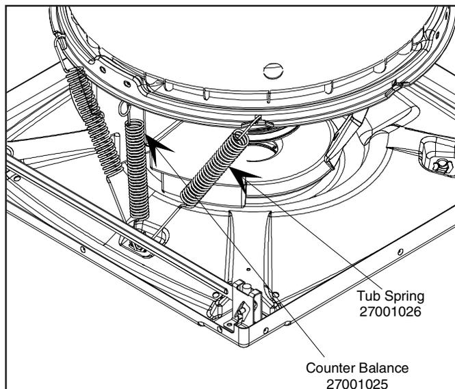
The 2 rear springs are mounted upsidedown to avoid the possibility of the springs rubbing together.
