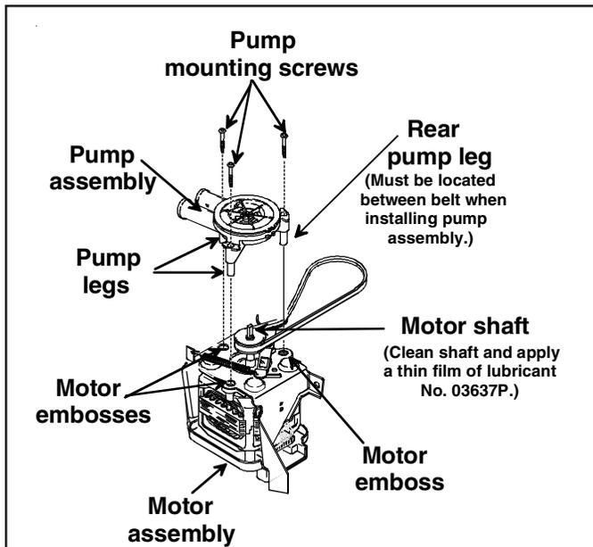
4. Align pump impeller hub with motor shaft. Verify belt encircles rear pump leg. Slide pump onto motor shaft until legs touch the embosses on the motor housing before securing.
