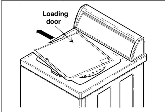
6. Remove screws securing right hinge and remove loading door.
