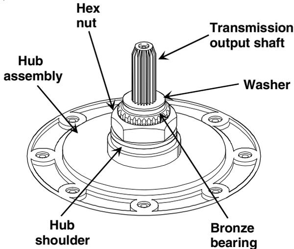
5. Clean all foreign material from seal mounting area of hub assembly, bronze bearing and washer.
