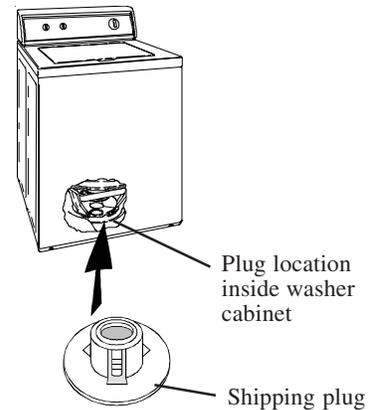
Refer to *Installation Instructions* for proper procedures whenever washer is moved.
