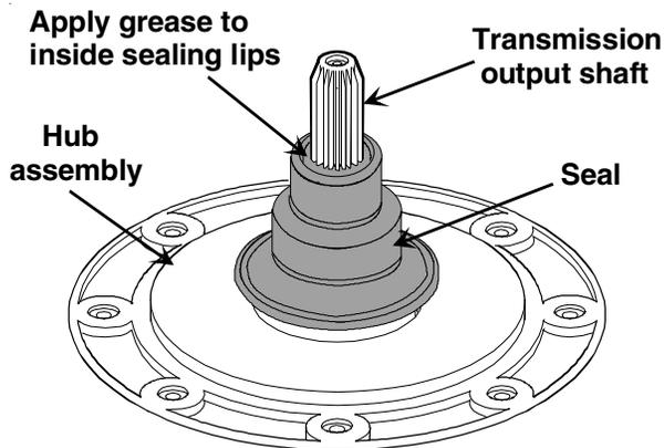
**NOTE:** DO NOT allow any lubricants to come in contact with outside surface of seal.
