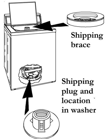
**Tilt washer back slightly and slide shipping plug into position under washer**
