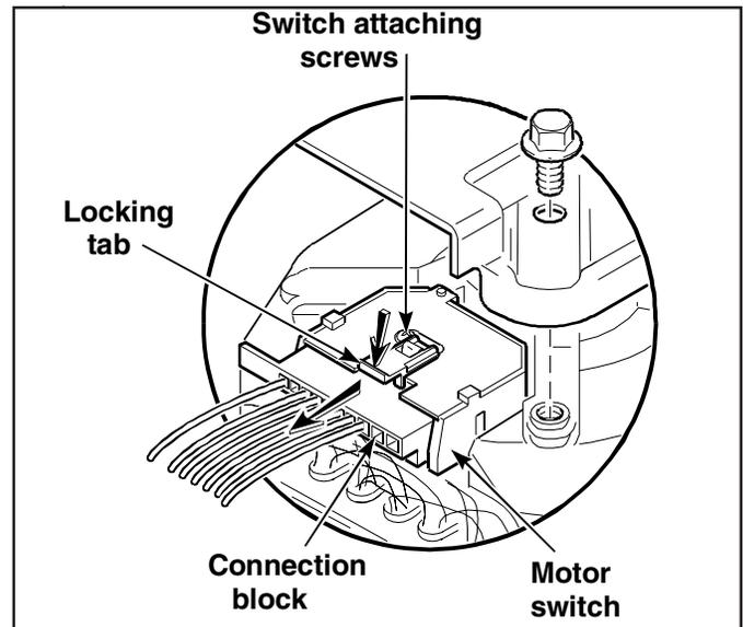
4. Remove screw securing motor switch to motor and remove switch.
