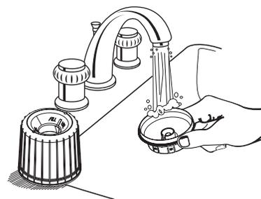
Clean funnel shape in top of agitator and inside of agitator. Use small brush on hole and slots in two funnel rings for thorough cleaning.
