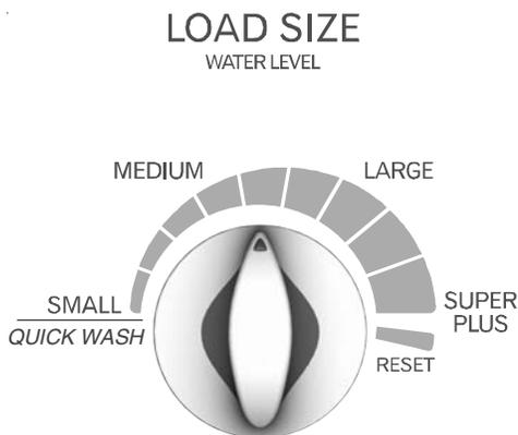
**IMPORTANT:** Do not hold knob at RESET for extended periods or washer flooding may result.
