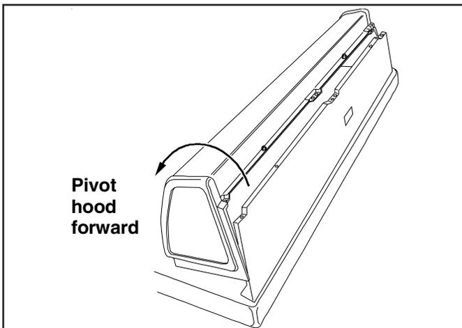
3. Remove bottom of control hood from clips located on cabinet top.
