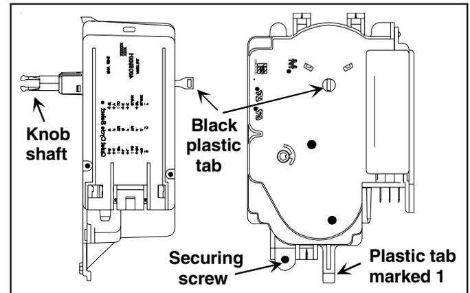
3. Remove screws securing timer to control hood mounting plate.
