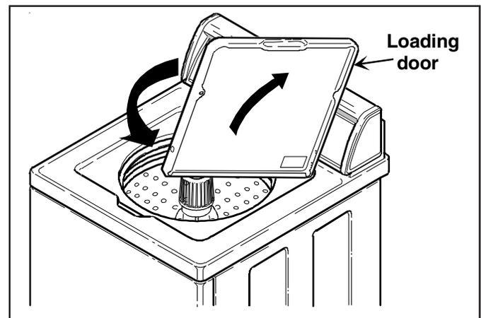
4. Rotate loading door so door is upside down.
