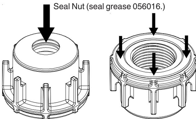
Seal Nut (seal grease 056016.)
