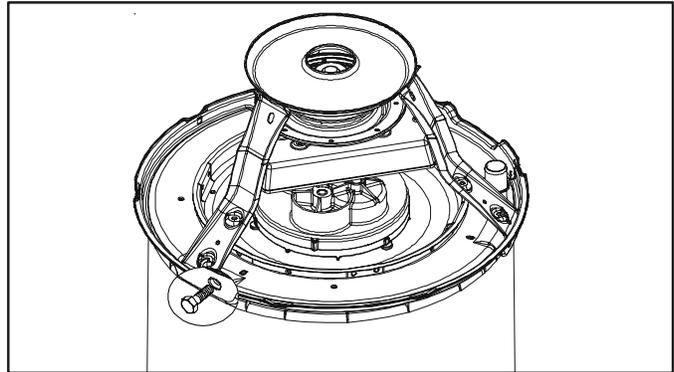
14. Remove seal and bearing using the brake removal tool 12002012 with included 3" PVC end cap.
