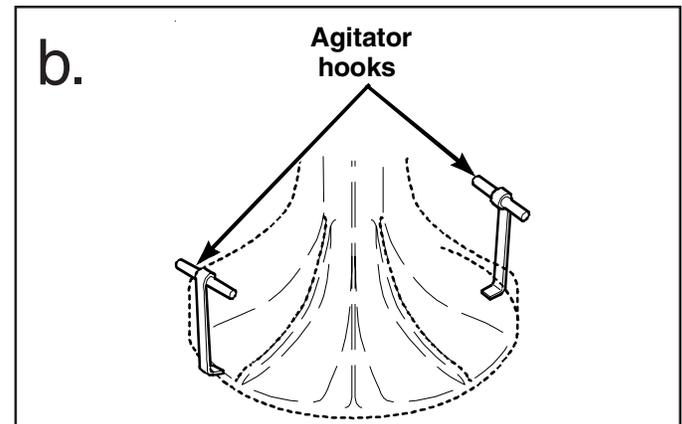
**NOTE:** Hooks must be positioned 180° from each other, and must be placed under base of agitator near agitator vane for greater stability. If hooks are placed between the vane area, agitator damage may occur.
