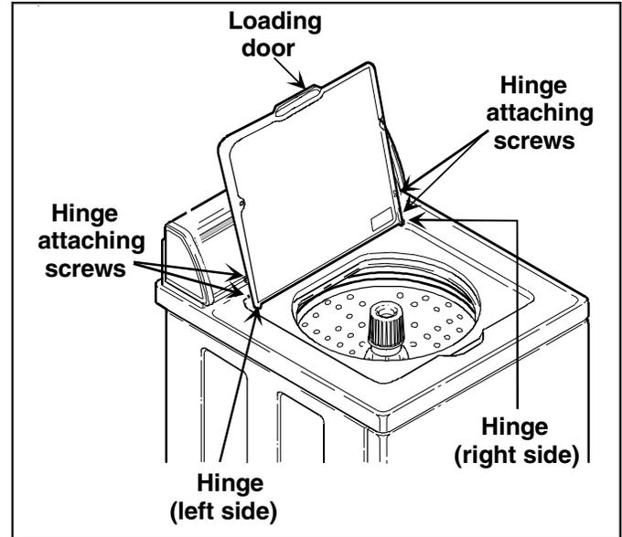
3. Raise loading door to a vertical position, disengage loading door from loading door clip by swing left side of door toward front of washer.
