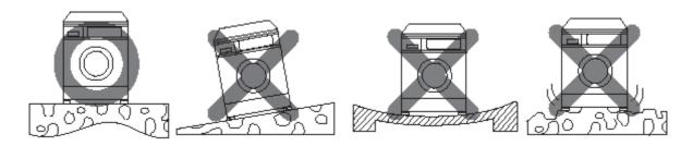
④ Adjust leveling with the leveling legs.
