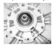
6. Separate tub front after removing 16 screws and suspension springs.
