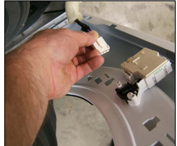
12. Disconnect door switch harness
