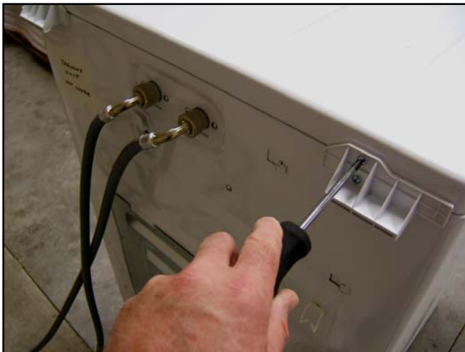
3. Remove 4 screws from rear
