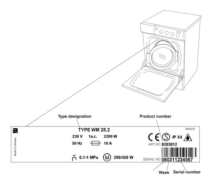
It should be easy to service a washing machine. It is important that you, as a service technician, are given the conditions to be able to carry out work in an efficient and satisfactory way. Our hope is that this service manual is a useful tool for your daily work.
