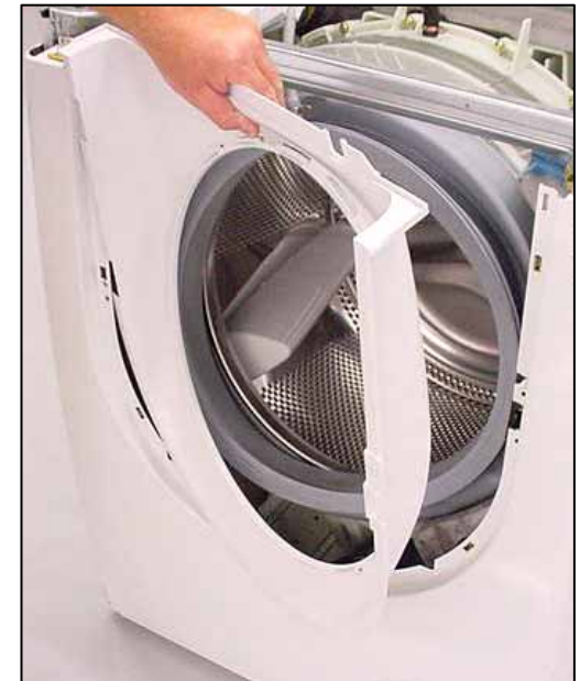
Removing front shield
