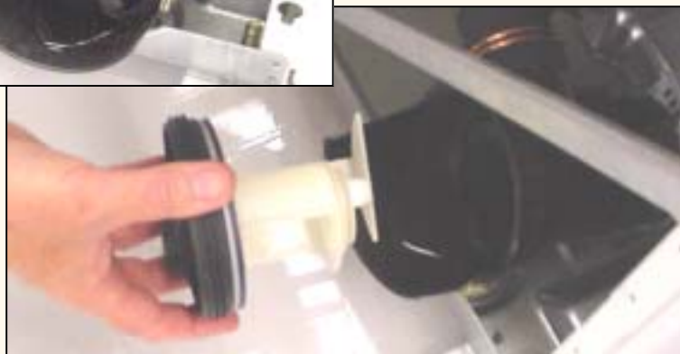
M3 Motor-Pumpe motor-pump 140 Ω... 200 Ω
