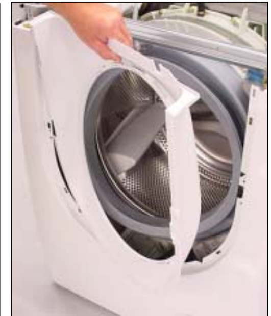
Removing front shield
