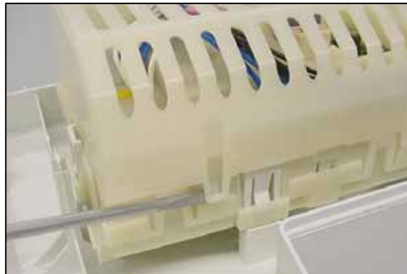
Pry outer & inner tabs together L – R
