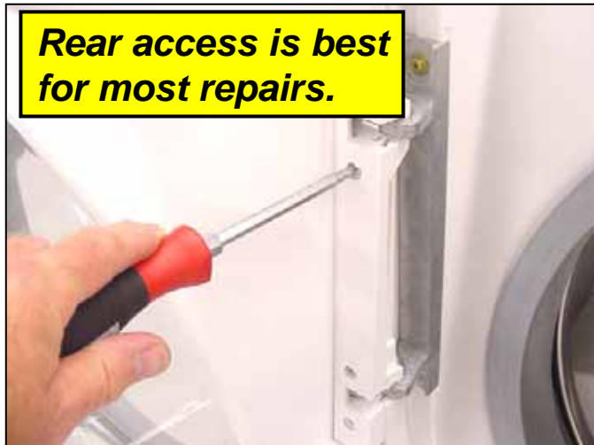
Remove hinge cover screws
