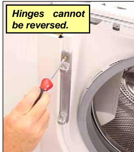
Remove hinge screws
