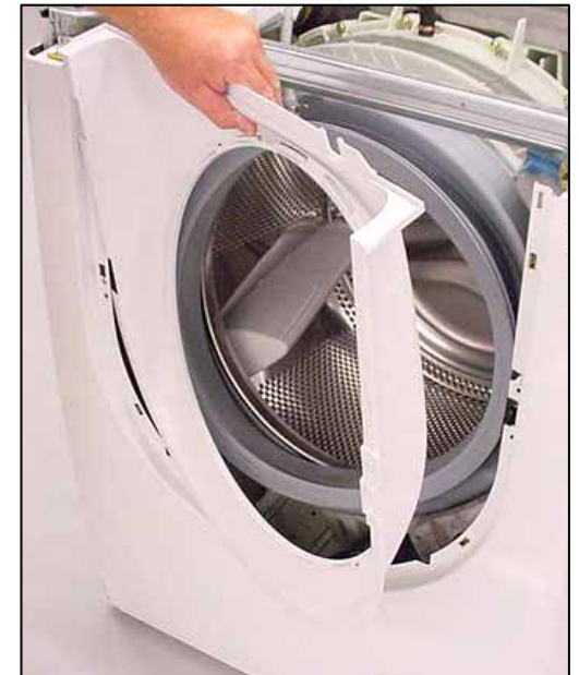
Removing front shield
