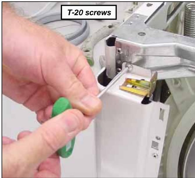
Remove top front panel screws
