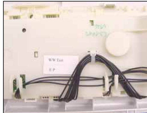
Pry outer & inner tabs together L – R
