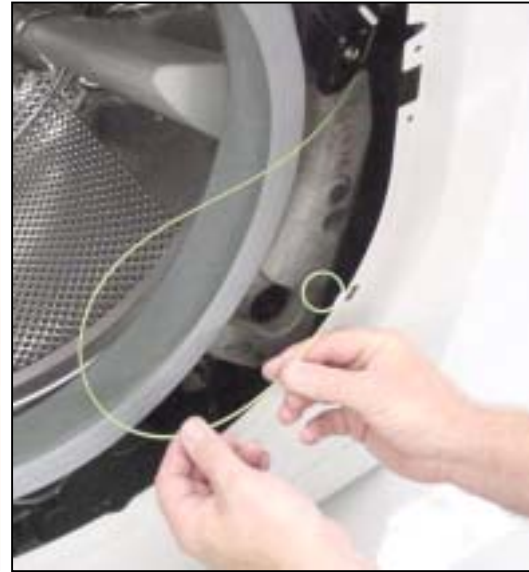
Note door latch manual release
