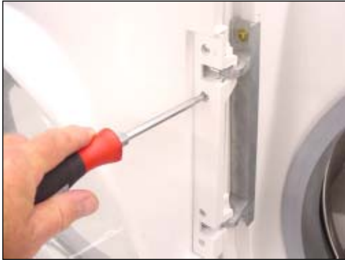
Remove hinge cover screws
