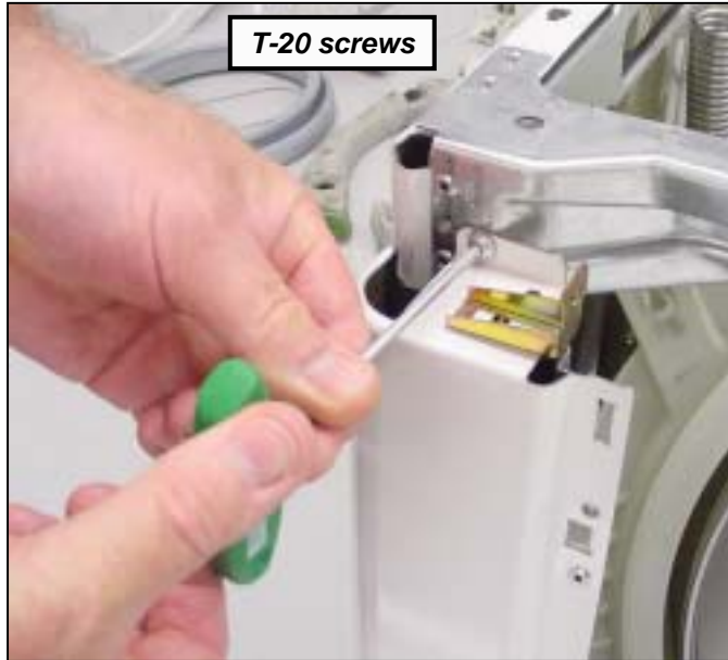
Remove top front panel screws
