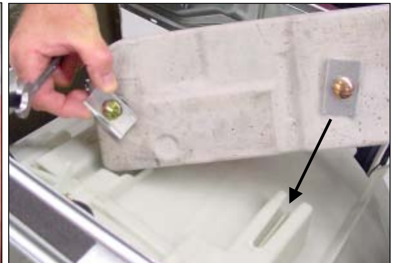
Note top counterweight bushing slots in tub
