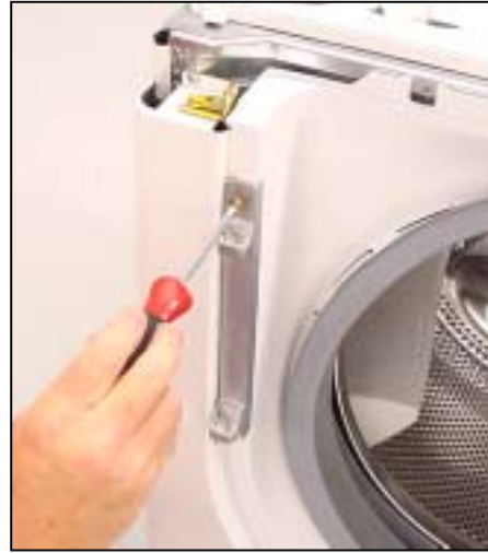
Remove hinge screws
