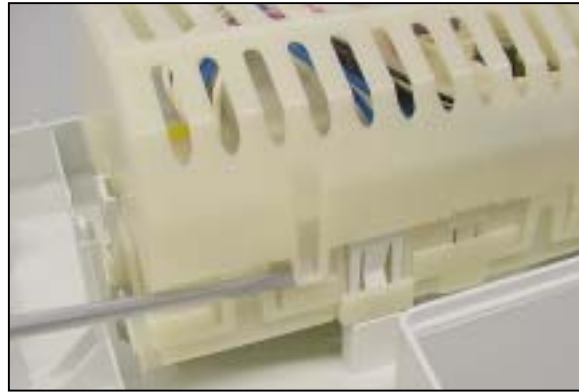
Pry outer & inner tabs together L – R
