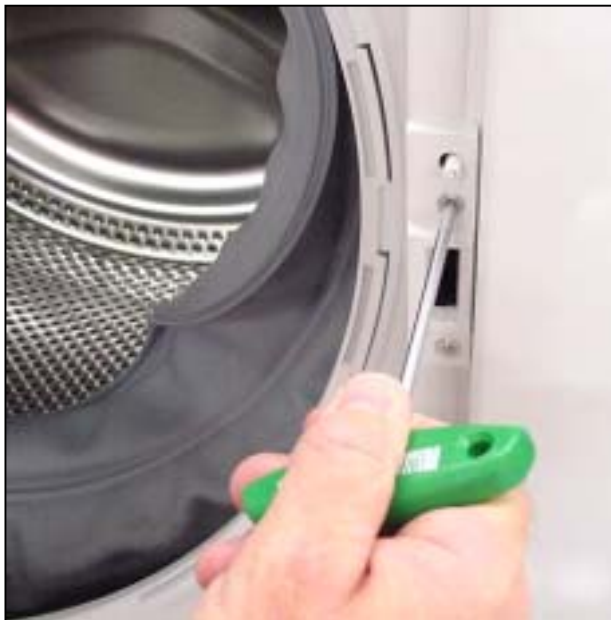
Remove door latch screws
