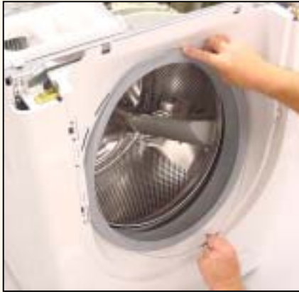
Remove front seal spring
