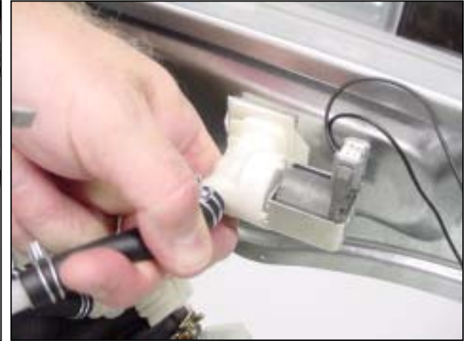
Disconnect hot water valve hose
