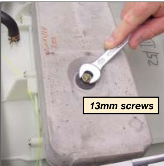
Loosen top counterweight screws
