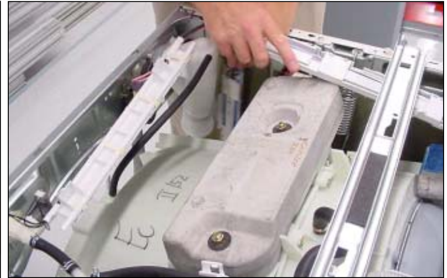
Top counterweight must be removed
