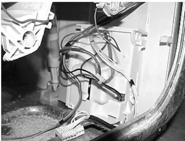
**Note:** The control board is the board that is mounted in the console and the speed control board is the board that is in the left rear corner of the washer.
