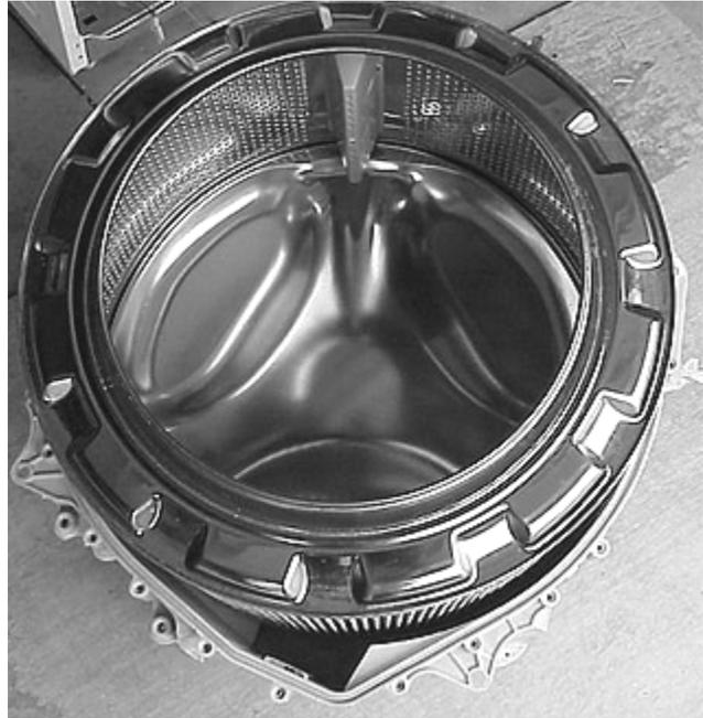
12. Turn the tub over and remove the (23) screws holding the two halves of the tub together.
