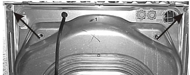
4. Pull back to disengage the (2) tabs and lift the brace off.
