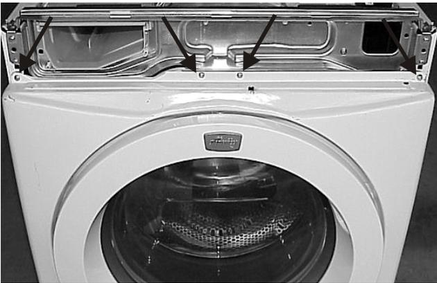
6. Lift up and out on the front panel to disengage it from the (4) nylon pins, two in the front of each side panel, and lift the front panel off.
