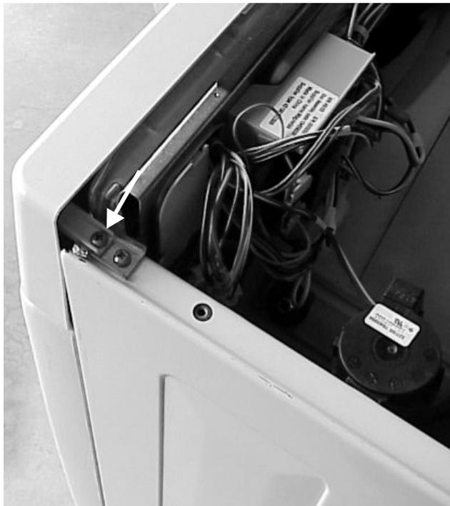
4. Lift the (3) tabs to release the top of console from the mounting plate.
