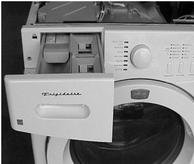
2. Push down on the release tab and pull the drawer out.
