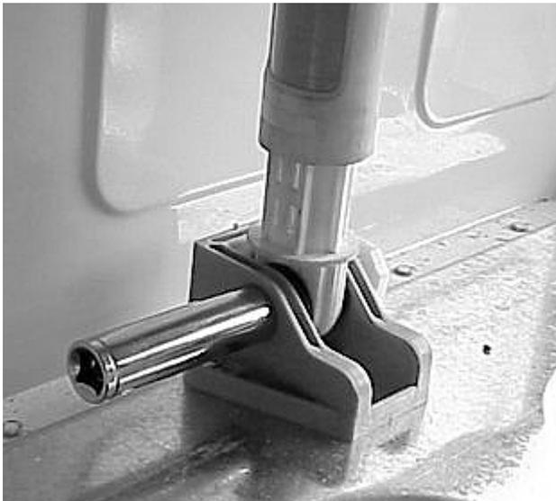
4. Use pliers to grasp head of pin and pull to remove. As the pin is removed the socket will drop free.
