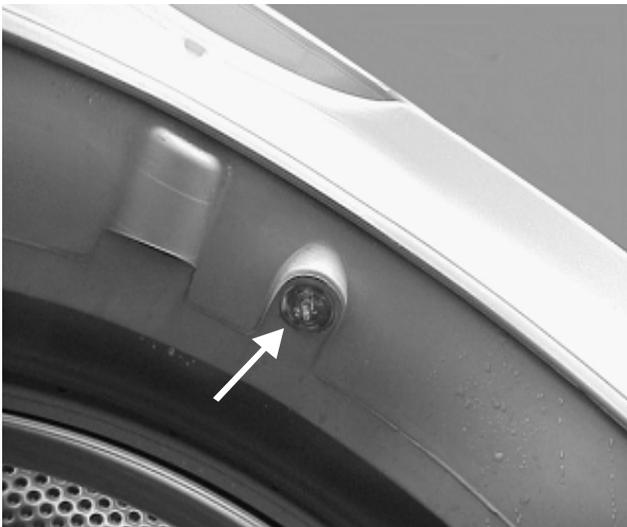
a pushbutton switch that is closed when the door is open,
