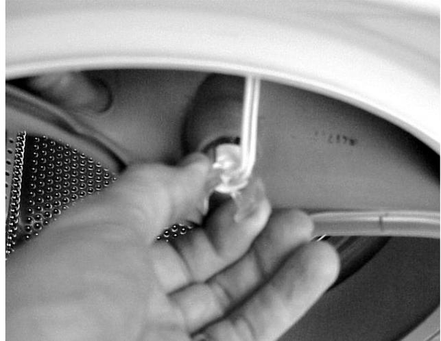
3. Release the (2) tabs on the dispenser drawer housing, one on each side housing and pull the bracket forward.
