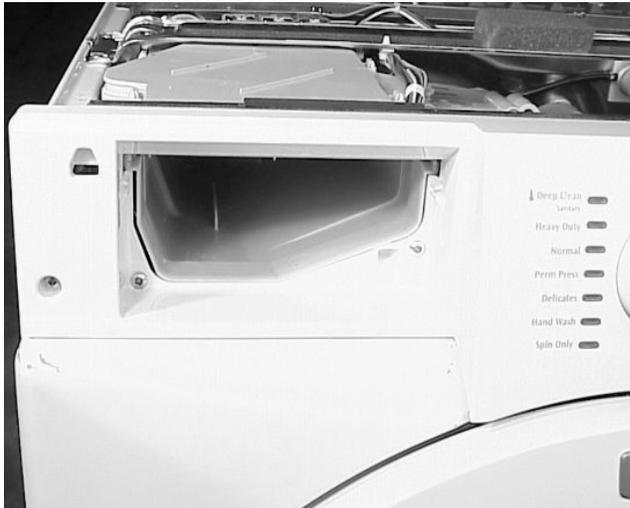
and a removable drawer with three cavities: one for detergent, one for bleach and one for fabric softener.
