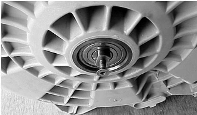
**Note:** The bearings, water seal and seal between the two tubs come as part of the rear half of the outer tub. If the water seal or bearings fail, inspect and if necessary dress the shaft of the spin basket with a file. With some failures, it may be necessary to replace the spin basket.
