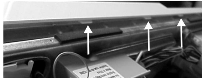
5. Roll the console forward, while lifting up to release the bottom tabs from the front panel.
