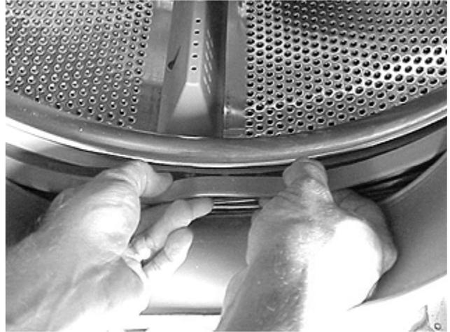
5. Using your thumb, start on the other side of the top tab and force the bellows on in the other direction. Again about one third of the way around stop and seat the bellows onto the tub lip. Force the remaining bellows on with your thumb and seat it.
