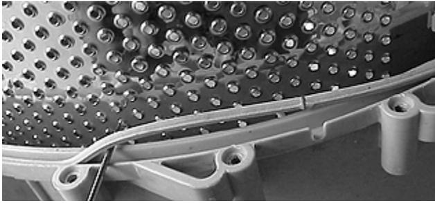
16. To remove the spin basket, set the back half of the outer tub on it's side, reinstall the screw that holds the large pulley on and tap the inner tub out with a rubber hammer.
