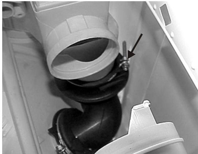
5. Remove the (2) screws holding the housing to the center brace.
