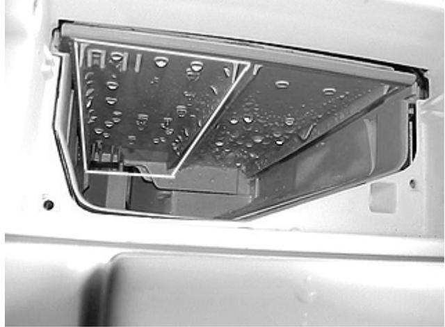
Since the flow of the incoming water is more than the holes can dispense, the excess water backs up into a channel across the rear of the dispenser.
