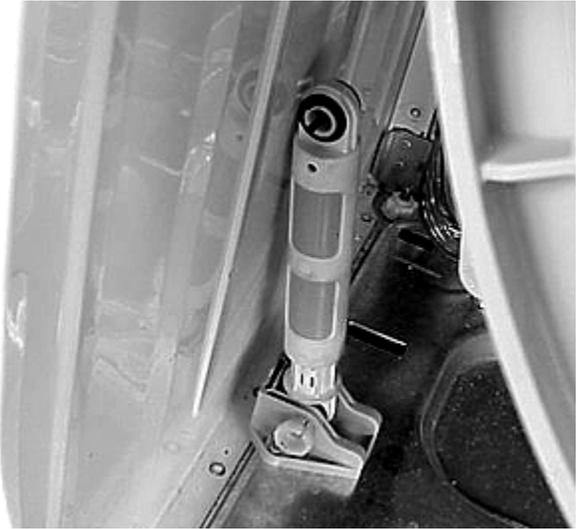
10. Place something down to protect the floor, carefully turn the washer on it's face and release the springs.
