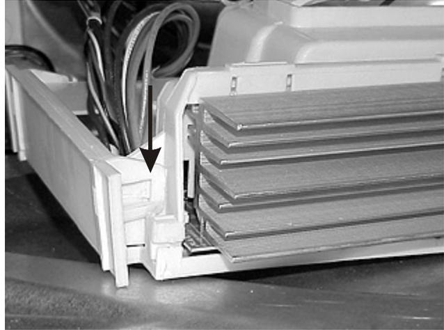
4. From the front of the washer tip the bottom of the assembly toward the motor and slide the assembly out between the shock absorber and the motor.
