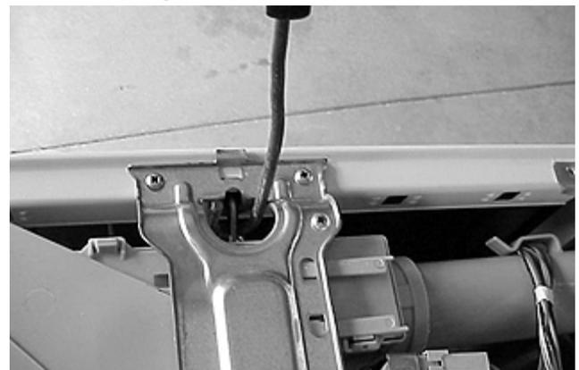
To do this a strong rod at least 8" long with a hook on one end and a handle on the other is needed, such as the one shown here made from a paint roller.
