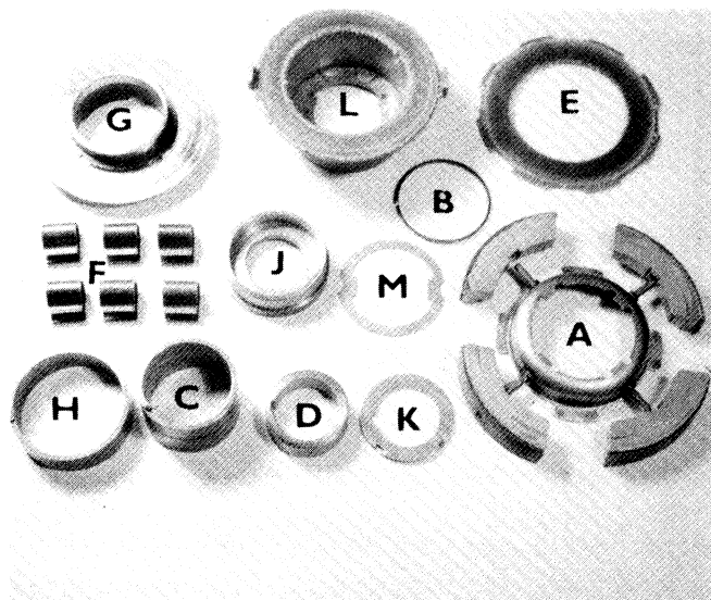
A. DECELERATOR SHOES AND MOUNTING BRACKET B. DECELERATOR SHOE BRACKET RETAINING RING C. CLUTCH TORQUE SPRING D. TORQUE SPRING COLLAR E. BRAKE PLATE F. BRAKE TENSION CLIPS
