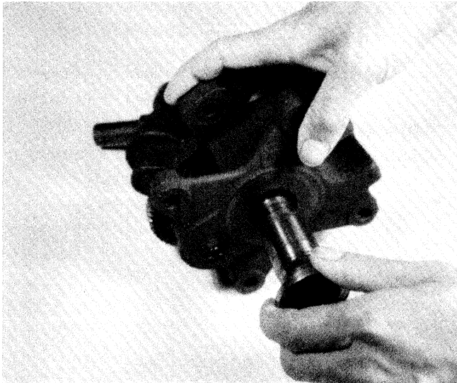
Figure 52 — Testing for Play in Drive Shaft and Spin Cage Base
