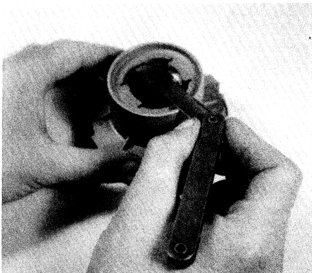
Figure 89 — Gaging Tolerance between Brake Spring Collar and Spacer Washer
