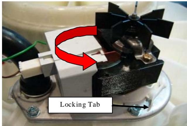
**Note: Approximately 1/3 gallon of water remains in the pump sump after pump out and will spill when the pump is removed. Take care not to spill this water over electrical connections by using a towel or small container to catch the water.**
