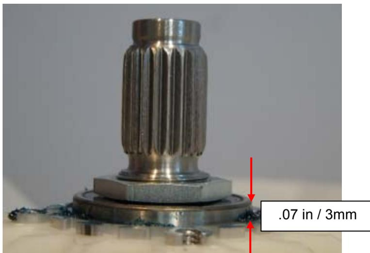
*Note: The outer bearing will be proud of the housing by approximately  $.07 \text{ in} / 3 \text{ mm}$ .*
