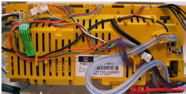
**Note:** When replacing a Motor Control Module ensure that the pressure tube is clear of any water droplets before operating the machine on a fill cycle. If the basket is full of water drain the water then blow down the tube before reconnecting the pressure tube.
