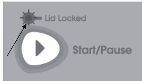
If the lid is left open, the machine will be unable to lock the lid and the cycle will be halted. The machine will play a tune and the lid lock will flash until the lid is closed and the **START/PAUSE** button is pressed.
