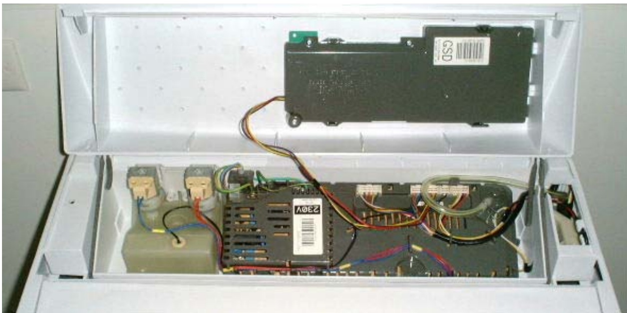
PHASE 5 TOPDECK SHOWING WIRING CONNECTIONS
