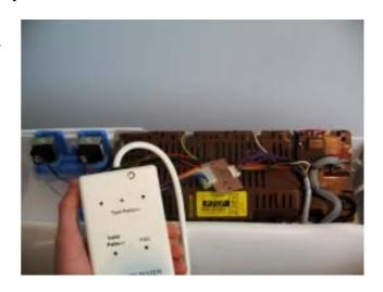
Note: This tester does not test all the functionality of the RPS. It tests the 3 outputs but cannot indicate all faults, for example if a capacitor on the RPS is cracked.
