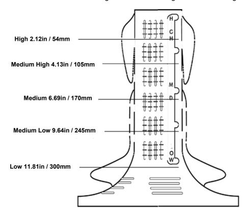
**EcoSmart® Water Level Settings**Tolerance for each water level = +/- .59in / 15mm
