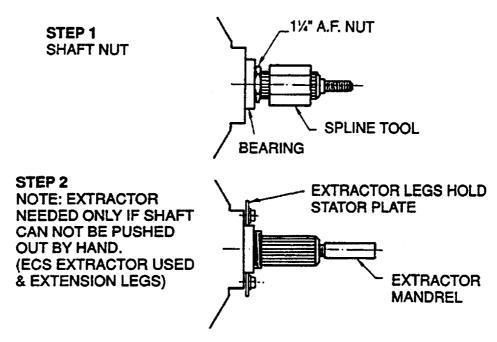
**WARNING**: Make sure the Stator clamp plate is flat before reusing. If in doubt, replace.
