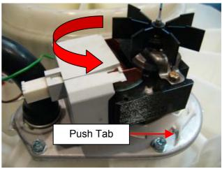
Note: Approximately 250mls of water remains in the pump sump after pump out and will spill when the pump is removed. Take care not to spill this water over electrical connections by using a towel or small container to catch the water.
