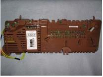
Note: When replacing a Motor Control Module ensure that the pressure tube is clear of any water droplets before operating the machine on a fill cycle. If the basket is full of water drain the water then blow down the tube.
