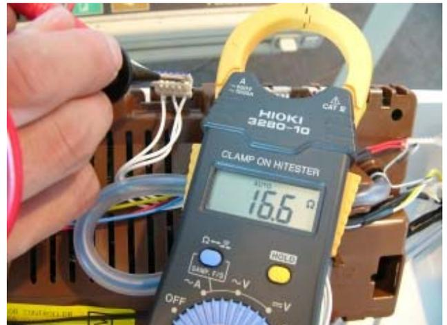
If the meter shows an incorrect reading, we would recommend testing the stator from underneath the machine, as there could be a fault in the wiring harness. To test the stator it will need to be removed from the machine (refer to Section 19.12).
