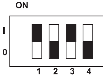
CORRECT SWITCH SETTINGS FROM FACTORY
