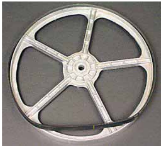
New Belt on Pulley
