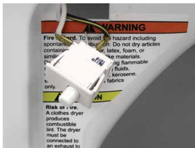
Door Switch (removed)
