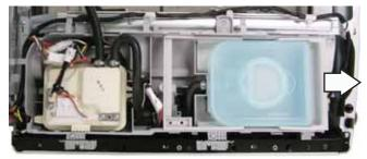
3. Disconnect the 2 hoses and the wiring harness from the water pump.
