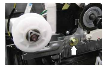
3. Remove the idler pulley by disconnecting the spring.
