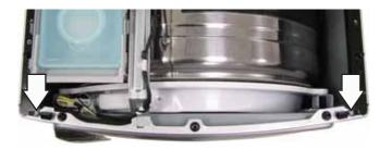
4. Tilt the front panel slightly forward to disconnect the wiring harness from the door switch.
