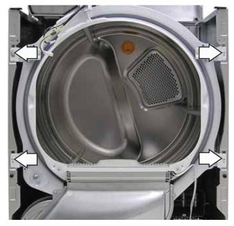
4. Remove the drum support by pulling straight out while dislodging the drum rollers.
