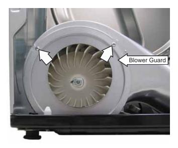
Note: In the following step, to prevent the blower wheel from turning while removing the center nut, apply a 7/8-in. wrench to the nut on the end of the drive motor.
