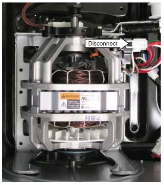
3. With a flat blade screwdriver, compress the open end of the spring strap (1 strap on each end of the drive motor) until it releases. Remove the spring straps.
