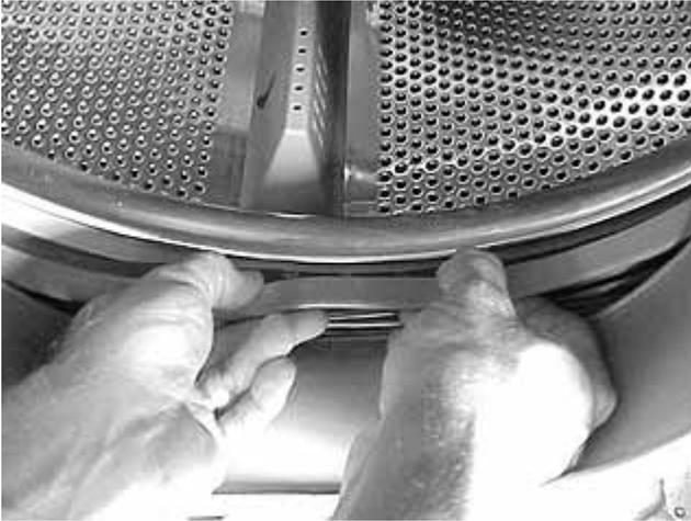
5. Using your thumb, start on the other side of the top tab and force the bellows on in the other direction. About one third of the way around, stop and seat the bellows onto the tub lip. Then force the remaining bellows on with your thumb and seat it.
