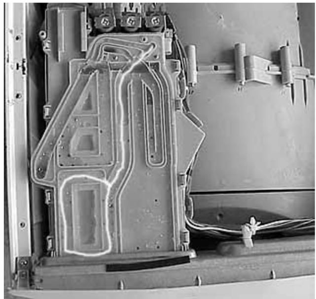
As the water passes over the detergent section, holes in the cavity allow some of the water to enter and flush the detergent cavity.
