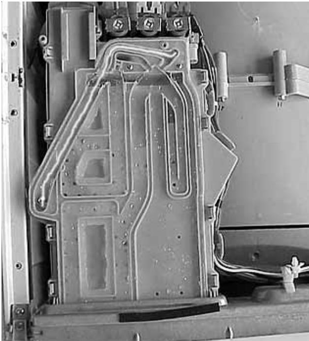
This path allows the water to bypass dispenser the drawer and enter the tub by a advanced rinsing technology hose connected between cavity and the bellows.
