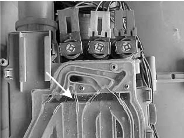
Detergent is dispensed at the start of the cycle, but bleach and fabric softener are not dispensed until later in the cycle. To allow all three items to be added to the washer before the start of the cycle, the bleach and softener cavities in the drawer have tubes molded into the bottom of them.
