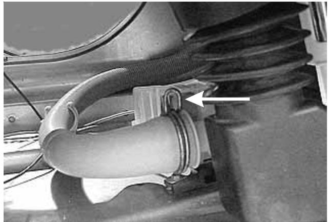
4. Remove the (2) screws, one on each side, holding the pump housing to the washer base.
