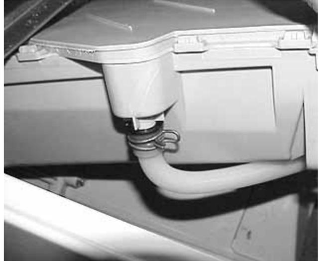
The detergent dispenser channel receives water from the right-hand input, as viewed from the front of the washer. The detergent channel forms a loop that allows the water to pass over the detergent section of the drawer.
