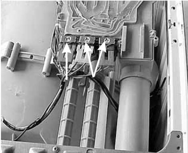
The hot and wash solenoids share a common output cavity, with the bleach solenoid having a separate output cavity.
