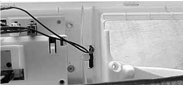
The reed switch contacts are controlled by the magnetic field of the magnet located in the front panel of the dispenser drawer.
