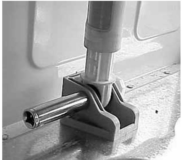
4. Use pliers to grasp head of pin and pull to remove. As the pin is removed the socket will drop free.
