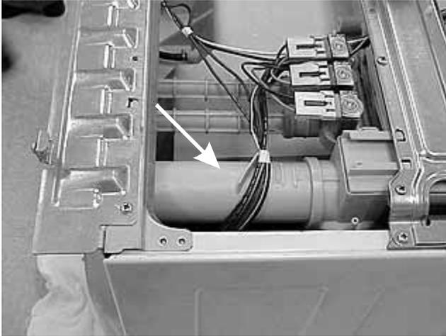
2. Turn the tube counterclockwise about a 1/16 of a turn to unlock the tube. Pull the tube back to disengage it from the detergent dispenser housing.
