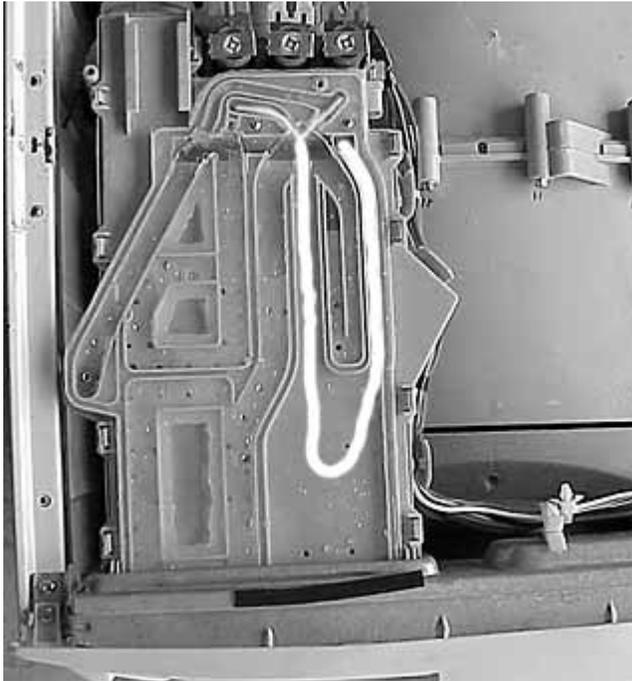
As the water passes over the fabric softener section, holes in the cavity allow some of the water to enter and mix with the fabric softener.
