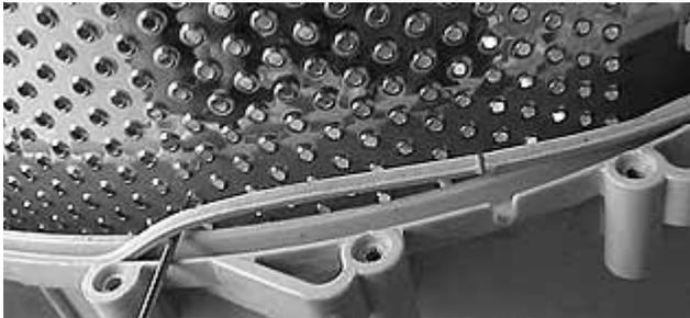
16. To remove the spin basket, set the back half of the outer tub on it's side, reinstall the screw that secured the large pulley to the shaft. Tap the inner tub out with a rubber hammer.
