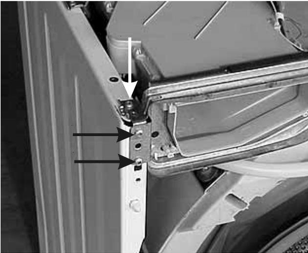
3. Release the (2) tabs on the dispenser drawer housing, one on each side, and pull the brace forward.
