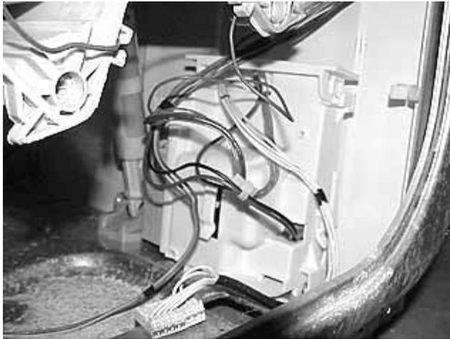
**Note:** The control board assembly is the board that is mounted in the console, and the inverter is in the left rear corner of the washer.
