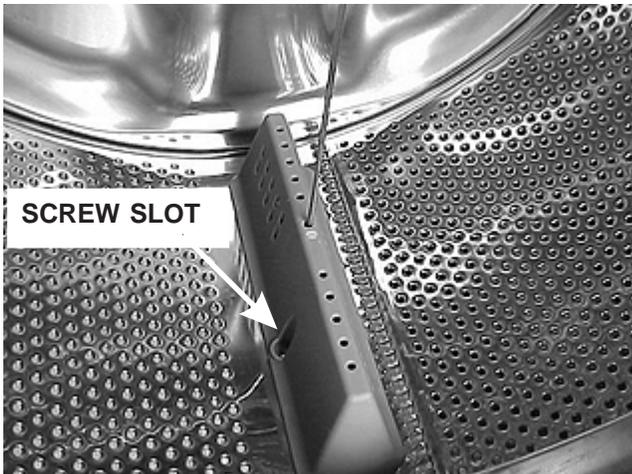
3. Slide the vane toward the door opening to release the (6) tabs and push on the side of the vane to remove.
