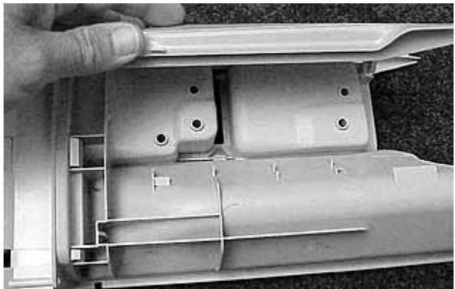
5. To remove the safety latch lever, compress the spring by moving the lever completely to the left and lift the lever out.
