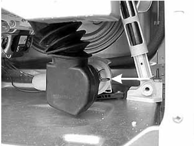
3. Release the clamp and slide the hose off the drain hose coupler.
