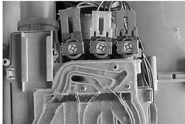
In the fill cycles, water enters into the top of cavity and is directed across the top of the cavity by 4 channels. The dispenser bypass channel, the detergent channel, bleach channel and the fabric softener channel. The channel that receives the water is determined by which inlet supplies the water or if both inlets supply the water.
