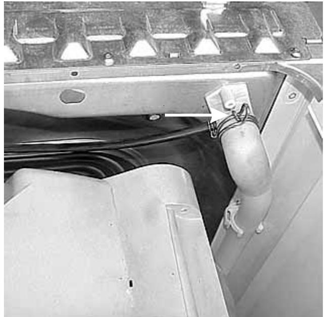
4. Slide the hose off of the tub and pump to remove the sump.
