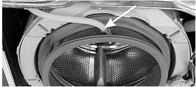
3. A groove in the rear of the bellows
