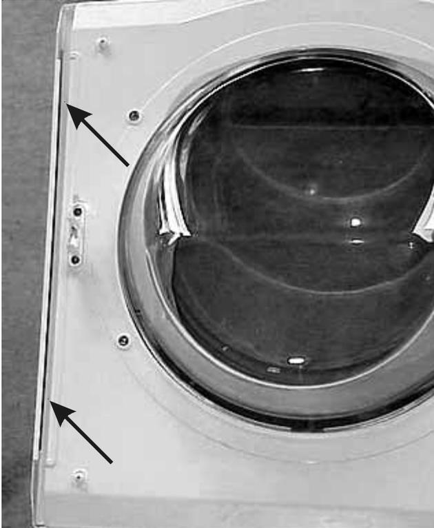
2. Remove the outer glass (some models) by removing the door strike and the (4) screws holding the outer glass to the inner panel and lift the glass off.
