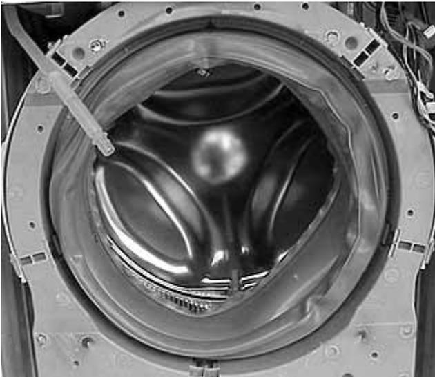
7. Place the spring in the groove at the top of the bellows and wedge a round object, about 3/4 " in diameter, between the weight ring and the bellows to hold the spring in the groove.
