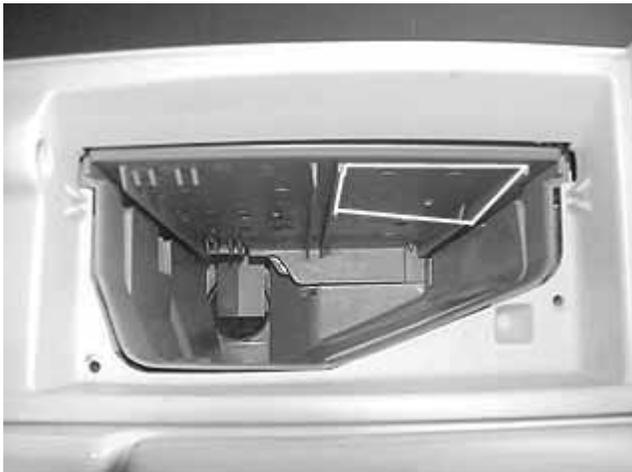
This raises the mixture level above the tubes in the drawer fabric softener cavity allowing the mixture to flow into the tub. Like the detergent channel, when the flow of the incoming water is more than the holes can dispense, the excess water backs up into the channel across the rear of the dispenser and flows into the tub.
