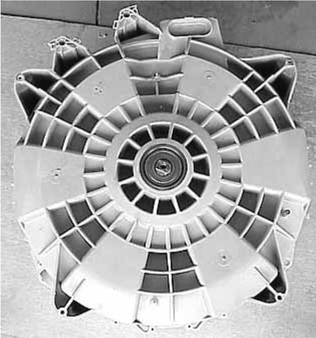
12. Turn the tub over and remove the (23) screws holding the two halves of the tub together.
