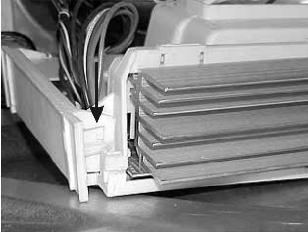
6. Unplug the (2) plugs and the ground wire and remove the speed control assembly from the washer.
