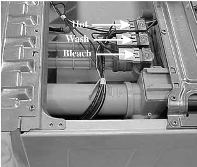
The hot solenoid is connected to the incoming hot water. The wash and bleach solenoids share a common input cavity that is connected to the cold water supply.
