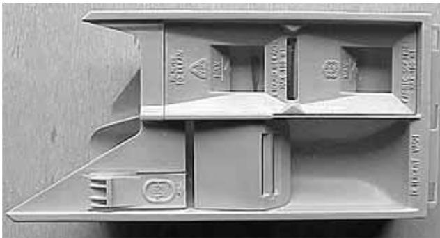
The inlet on the left, as viewed from the front of the washer, is connected to the left-hand cold water solenoid.
