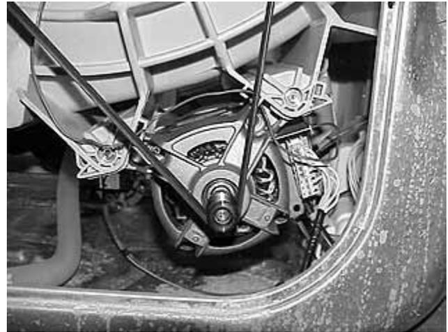
The motor is an induction, three phase AC motor that varies speeds when the voltage from the speed control board varies in frequency and amount. The motor has a tachogenerator that inputs the speed of the motor to the speed control board.
