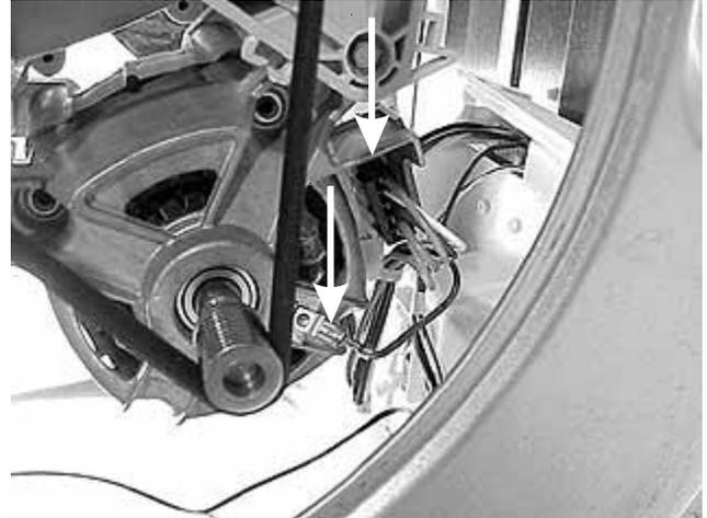
3. Using a 5/16" socket, remove the (4) bolts, two in the front and two in the rear, that secure the motor to the outer tub.
