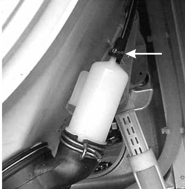
3. Release the rivet holding the air bell to the outer tub.
