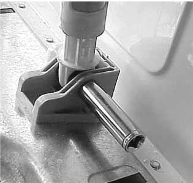
5. Use pliers to grasp head of pin and pull to remove. As the pin is removed the socket will drop free.
