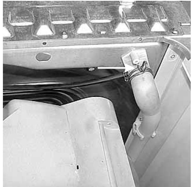
4. Slide the hose off of the tub and pump to remove the sump.
