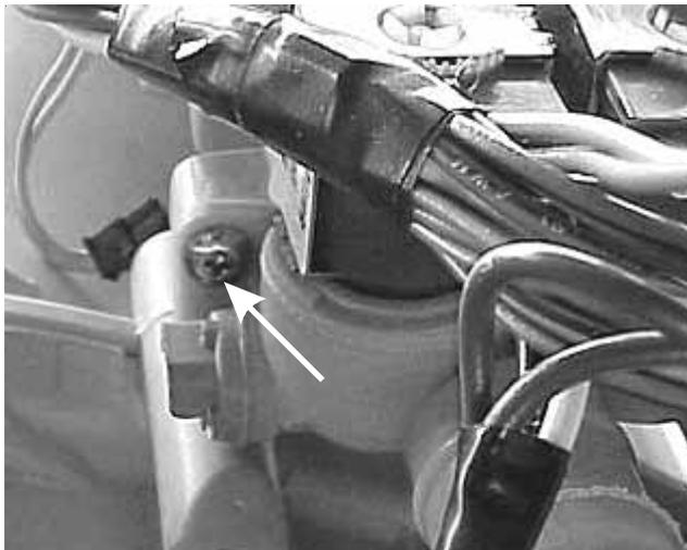
5. Pull back on the valve assembly to disengage it from the detergent dispenser housing and lift out.
