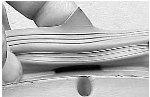
3. Place the slot over the tab and, while holding the bellows in place with one hand, place the other hand inside the bellows and force the groove of the bellows over the lip of the tub with your thumb.
