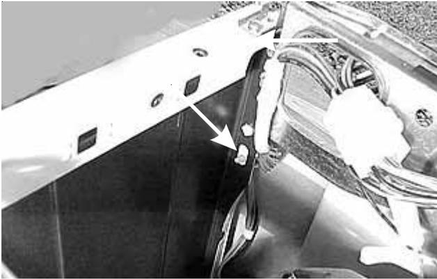
4. Remove the (3) screws holding the front panel to the front console mounting brace and side panels.
