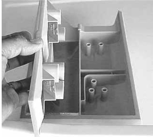
3. To remove the drawer front, release the three tabs and pull the drawer front away from the body.
