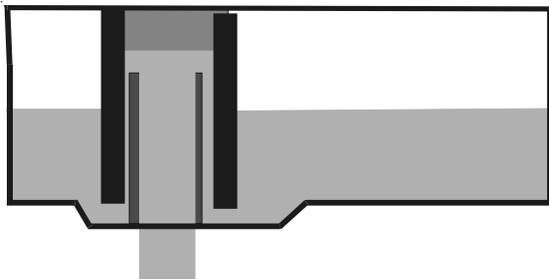
The bleach dispenser channel receives water from the left-hand input, as viewed from the front of the washer. The bleach channel forms a path that allows the water to pass over the bleach cavity section of the cavity.
