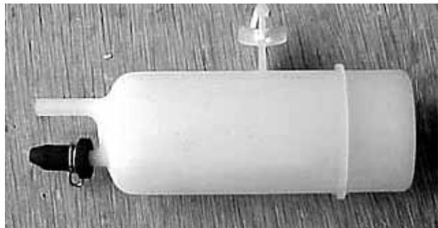
**NOTE: Seal air connecting tube to air bell and air bell to sump hose using waterproof glue. DO NOT plug air connecting tube opening.**
