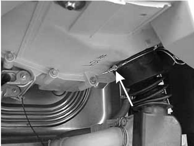
2. Release the clamp and slide the hose off the drain pump.
