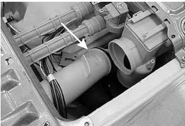
4. Drop the rear of the tube down, slide the tube back and lift the tube out.
