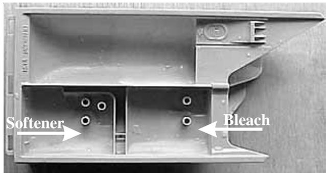
These tubes allow bleach or softener to be added to their cavity without being dispensed as long as the liquid is below the top of the tubes. At the proper time in the cycle, when bleach or fabric softener is to be dispensed water is added to the cavity. This raises the mixture above the top of the tube and the bleach or fabric softener starts flowing into the tub.
