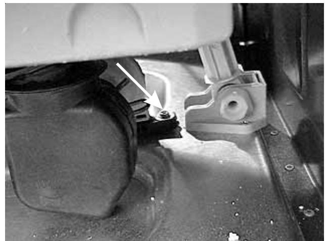
4. Unplug the wires from the pump motor.
