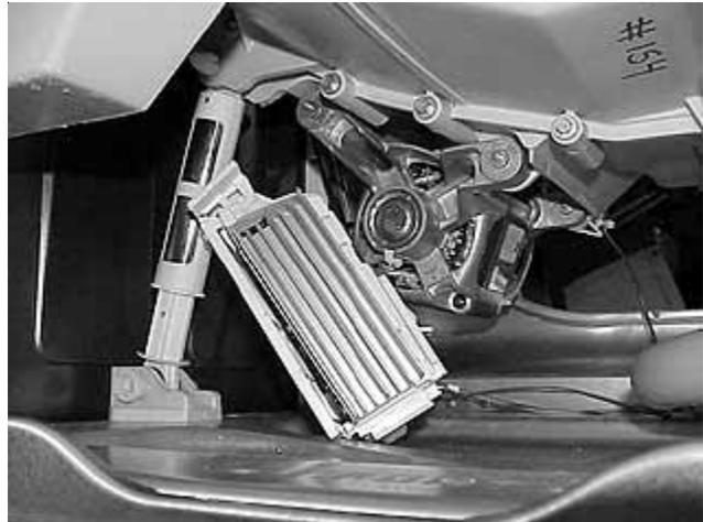
5. Release the latch on each end of the speed control housing and raise the top flap.
