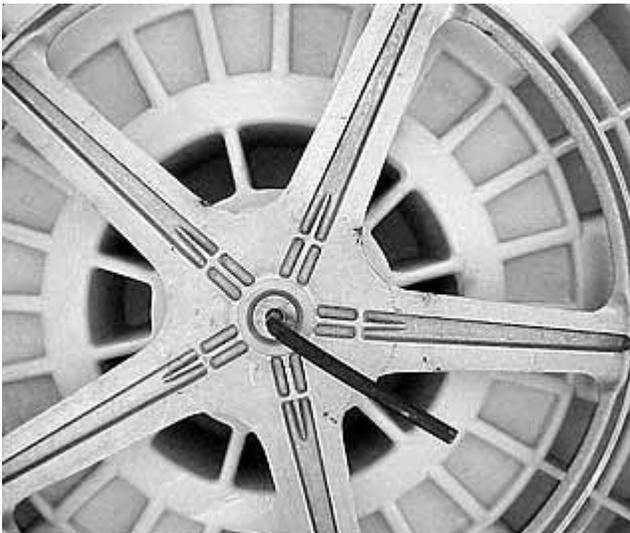
4. Work the pulley back and forth to remove it from the shaft.
