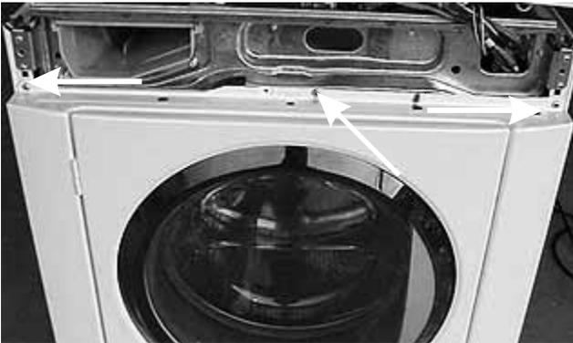
5. Remove the (2) 5/16" hex head screws holding the bottom of the front panel to the side panels.
