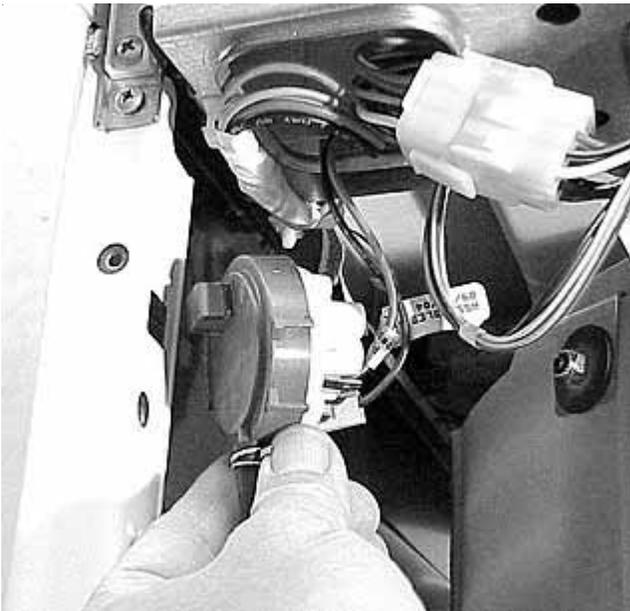
4. Disconnect the hose from the pressure switch.
