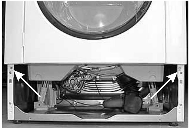
6. Lift up on the front panel to disengage the (2) pins (one in each side panel) the front panel hooks over.
