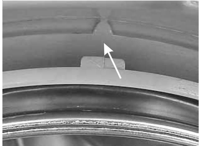
and a slot in the groove and an arrow at the top of the bellows.
