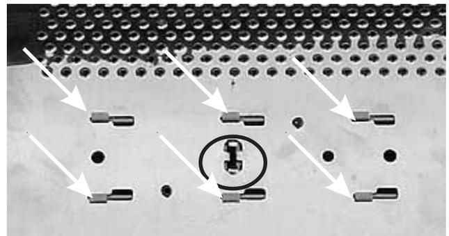
Each vane is locked in place by (4) tabs pressed out of the spin basket.
