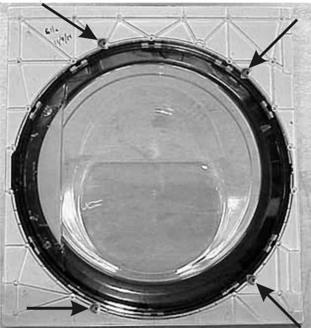
3. The inner glass is held in place by (5) molded tabs in the rear door cover. To remove the glass, grab the edge of the cover by the tab and twist it away from the glass.
