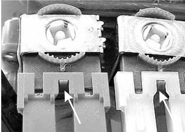
4. Remove the (2) screws, one on each side, holding the water inlet valve assembly to the detergent dispenser housing.
