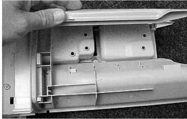
The 2 outlets of the water inlet valve assembly are inserted into the rear of the automatic dispenser. During the fill cycles, water is directed into the top of the cavity through 2 inlets. The inlet on the right, as view from the front of the washer, is connected to the combination output of the hot water solenoid and the center cold water solenoid.
