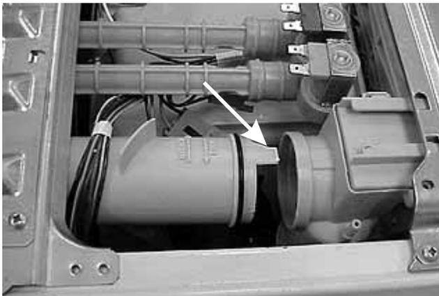
3. Push the front of the tube down and forward toward the water inlet valve assembly until the tube clears the rear panel.
