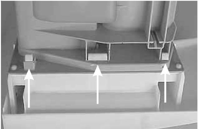
4. To remove the conveyor, release the conveyor from the tabs and lift it off.
