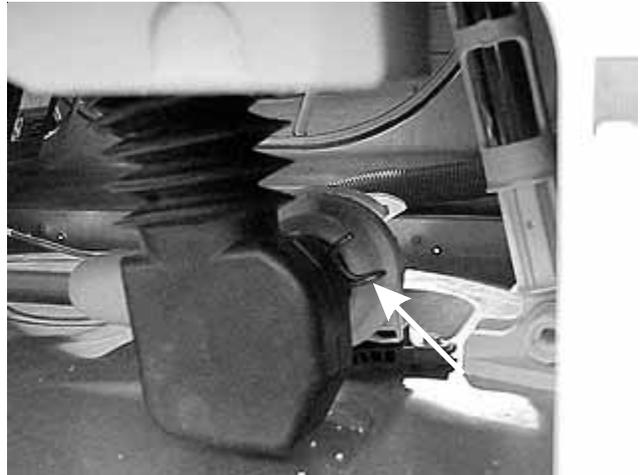
3. Disconnect the outlet hose from the pump.
