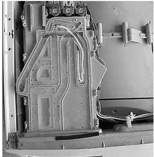
As the water pass over the bleach section, holes in the cavity allow some of the water to enter and mix with the bleach.
