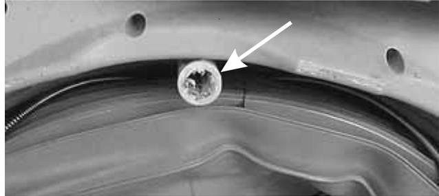
8. Pull the spring with one hand while working it into the groove with the other.
