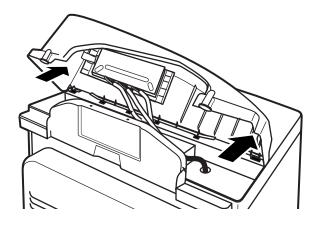
17. Secure the new backsplash to the dryer using the 4 Phillips head screws removed earlier.
