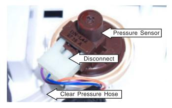
The pressure sensor wires (purple, orange, and blue) are connected at pins 1, 3, and 4 at the 4-pin red connector on the inverter board. (See *Inverter and Main Board Pin Connectors*).
