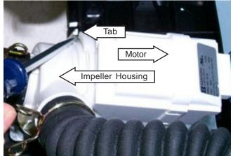
5. Remove any foreign objects from the impeller and impeller housing. Inspect the impeller for any damage and replace the pump assembly if necessary.
