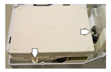
3. Lift the inverter box up. Press the tabs on the side and gently pry it open.
