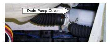
4. Remove the drain hoses from the pump:
