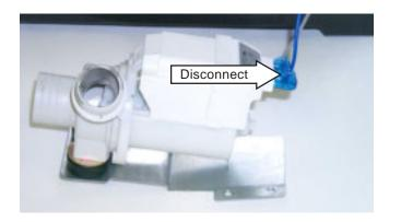
7. Remove the 2 Phillips head screws that hold the drain pump to the mounting plate. Remove the drain pump.
