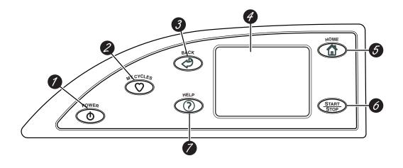
Features of the washer control panel 1 **POWER.** Press to "wake up" the display. If the display is active, press to put the washer into standby mode. You may also press the Touch Screen or any button to "wake up" the display.
