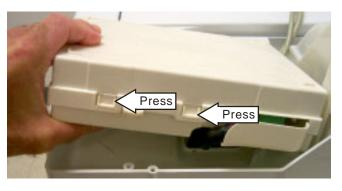
4. Disconnect the wiring from the inverter board. Remove the inverter.
