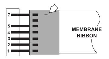
**Note:** The number (1) molded on the membrane connecter is not a pin reference number.
