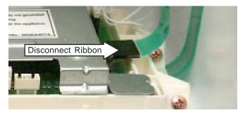
Remove the 4 Phillips head screws (2 on each side) that hold the main control board and LCD touch screen assembly in place. Remove the assembly.
