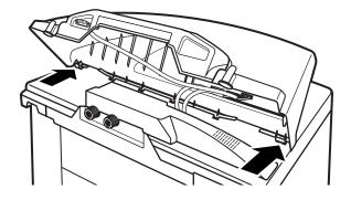
23. Secure the new backsplash to the washer using the 2 Phillips head screws removed earlier.
