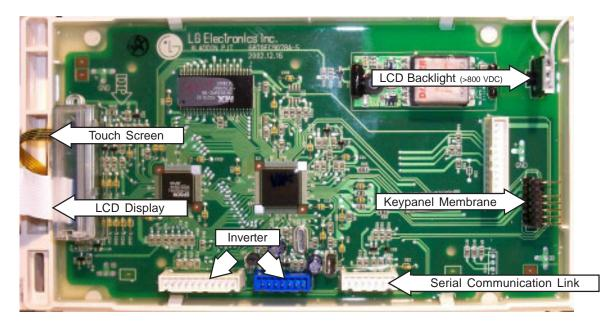
WARNING: THE CONNECTOR AT THE LCD BACKLIGHT IS OVER 800 VDC. USE APPROPRIATE TYPE VOLTMETER OR DAMAGE COULD RESULT.
