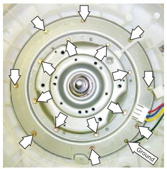
4. Remove the bearing housing assembly.
