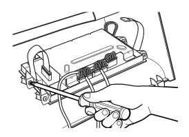
21. Place the gray wire from the serial port under the strain relief of the new backsplash.
