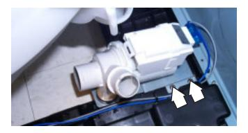
6. Disconnect the drain pump wires.
