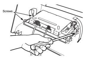
14. Connect the dryer control board to the new backsplash by sliding the ribbon connector on the new backsplash onto the metal pins on the control board and pushing in. Make sure the ribbon is not twisted before inserting the connector.
