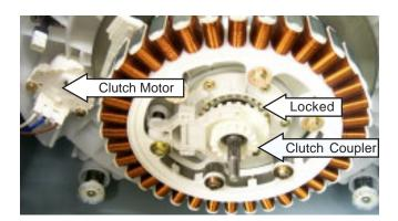
• When the basket and infusor are in the unlocked position, the clutch moves upward, disengaging the clutch coupler and rotor teeth, allowing the infusor to rotate independently of the basket.
