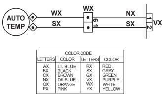
THE "X' INDICATES ONE SOLID COLOR-NO TRACER. WIRES WITH TRACER SHOW BOTH COLORS, EXAMPLE - WR IS WHITE WITH RED TRACER. Resistance can be measured at the purple 2-pin connector on the inverter board. Make sure to unplug the connector to isolate the thermistor before taking resistance readings. (See *Inverter and Main Board Pin Connectors*.)
