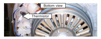
To determine the temperature of the incoming water, the washer control measures the difference between the voltage sent and the voltage returned from the water temperature sensor. The washer control then makes temperature adjustments accordingly.
