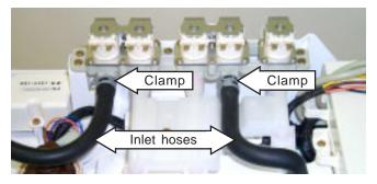
5. Remove the 3 Phillips head screws that hold the water valve assembly in place and the 2 Phillips head screws that hold the water distribution pipe in place.
