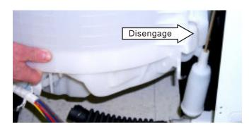
4. Pull the outer tub assembly out of the washer cabinet.
