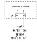
To determine the temperature of the incoming water, the main control measures the difference between the voltage sent and the voltage returned from the thermistor. The main control then makes temperature adjustments accordingly. The main control should fill the tub with water within +/- 10 to 15°F of set temperature by opening or closing the hot and cold water valves.
