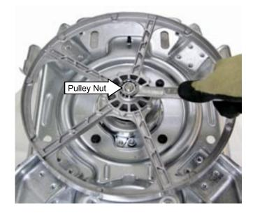
**Note:** When replacing pulley, tighten pulley nut to 275 in. lbs. of torque.
