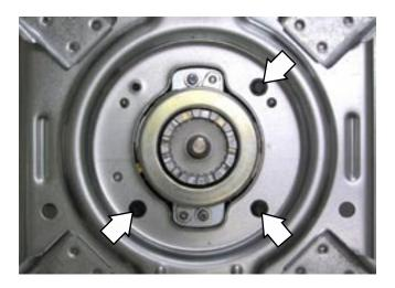
9. Remove the four ½-in. hex-head bolts that attach the platform to the tub.
