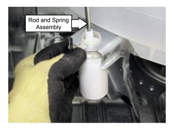
Note: The tub assembly will now lean forward. This allows clearance to reach behind the tub and access the rear rod and spring assemblies.
