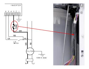
If the fuse is open, agitate, spin, and mode shifting does not occur. Check the fuse connections and wiring harness.
