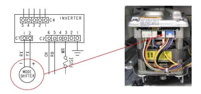
**Note:** The mode shift coil connects to C7 connector on inverter/motor assembly. Unplug C7 connector and check continuity. Mode shift coil resistance value is approximately  $98\Omega$  @ room temperature (77° F).
