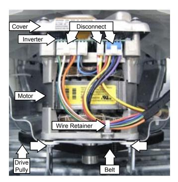
**Note:** Minimal clearance exits between the 2 rear <sup>3</sup>/<sub>4</sub>-in. motor nuts, isolators, and the drive pulley.
