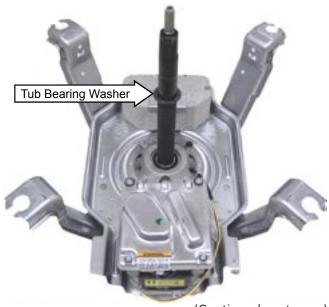
12. Remove the inverted single <sup>3</sup>/<sub>8</sub>-in. hex-head bolt from the top of the platform.
