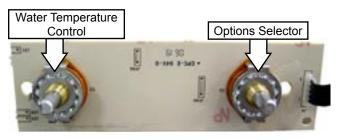
**Note:** The water temperature control and the options selector have detents between some of the settings. The washer will function if the knob is inadvertently set at one of the unmarked detents. Following a clockwise direction, all unmarked detents have the same value as the marked detent before it. The highlighted areas below show an example of what settings would be selected.
