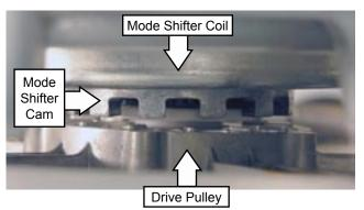
Note: Mode shifter coil energized for agitate mode; cam teeth disengaged from drive pulley.
