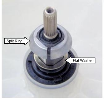
Note: A new seal (part number WH02X10032) is included with a replacement tub or shaft and mode shifter assembly. Replace the seal when the tub has been separated from the shaft and mode shifter assembly.
