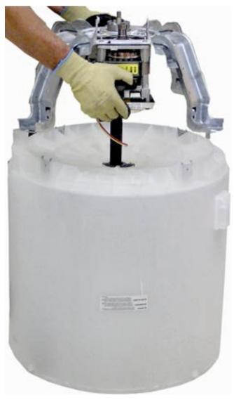
11. Place the platform upright on a protected surface and remove the tub bearing washer from the tube.
