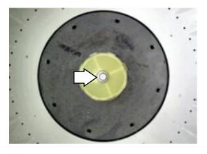
**Caution:** Use only a rubber mallet, dead blow hammer, or impact wrench to remove the hub nut. Use of a steel head hammer may result in damage to the spin basket.
