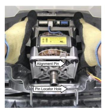
**Note:** When replacing a motor, check its brake operation. Place washer in a spin cycle and lift the lid after it has reached full speed. The basket should stop within 7 seconds. If time exceeds 7 seconds check the lid switch operation, and check the belt for worn ribs or slippage due to residue on the belt or pulleys.
