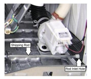
The shipping rod passes through the chassis rod brackets and the platform brackets.
