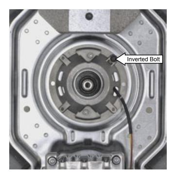
13. Lift the shaft and mode shifter assembly from the platform.
