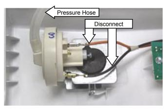
5. Press the plastic locking tab, rotate the switch counterclockwise, and pull the switch out of the control panel.
