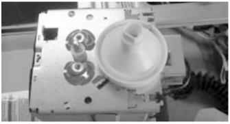
All other selector knobs are D-shaped and can be removed by pulling straight out.
