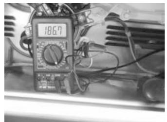
With volt/ohmmeter probes attached to the right and center leads, the reading should approximate the one in the picture. With a required resistance of 184 ohms, this reading is within the acceptable range. The information is provided in the schematic. Remember to access the tachoenerator leads from the front.
