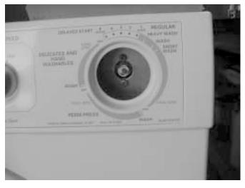
Timer motor resistance is approximately 2.4K ohms +/- 7%. (See Resistance Chart or Schematic for resistance values.)
