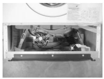
With the front panel removed, and the motor connector exposed, you can check the motor windings. They are color coded in the schematic as black, blue, and red.
