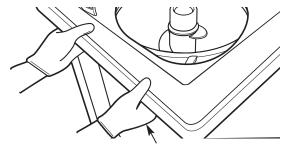
Locate hooks in cover slot; squeeze against apron bracket to engage.
