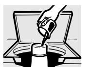
The fabric softener dispenser automatically releases liquid fabric softener at the proper time during the cycle.
