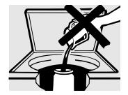
Do not pour anything into the agitator if the agitator cap or dispenser is removed.
