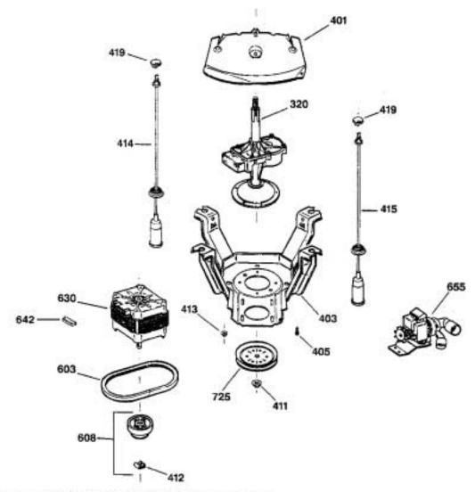
NOTE: REF. 412 (WH1X2733) SHOULD BE REPLACED EACH TIME CLIP IS REMOVED.
