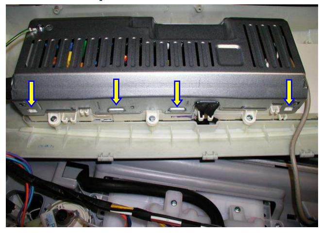
To remove metal shield from control board assembly, pull outward on side tabs.
