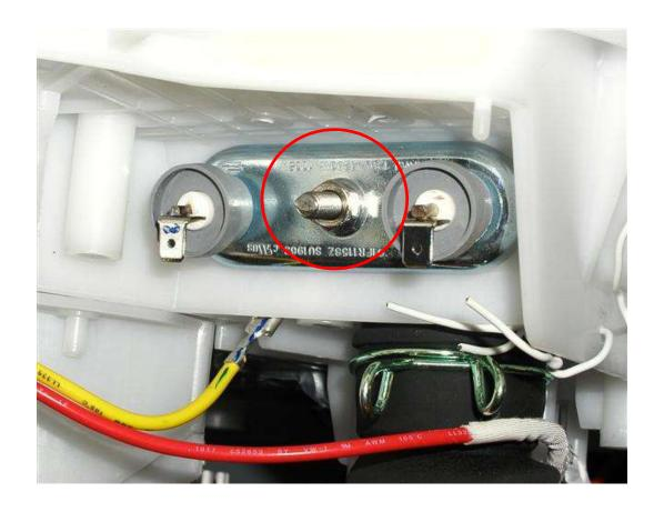
**CAUTION:** Proper torque must be applied to the 10mm hex nut in order to assure a proper seal.
