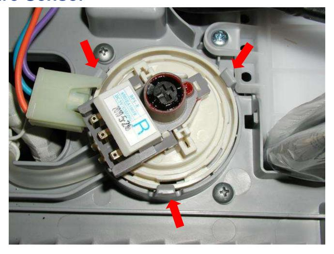
Sensor is held in place by three flexible, plastic tabs.
