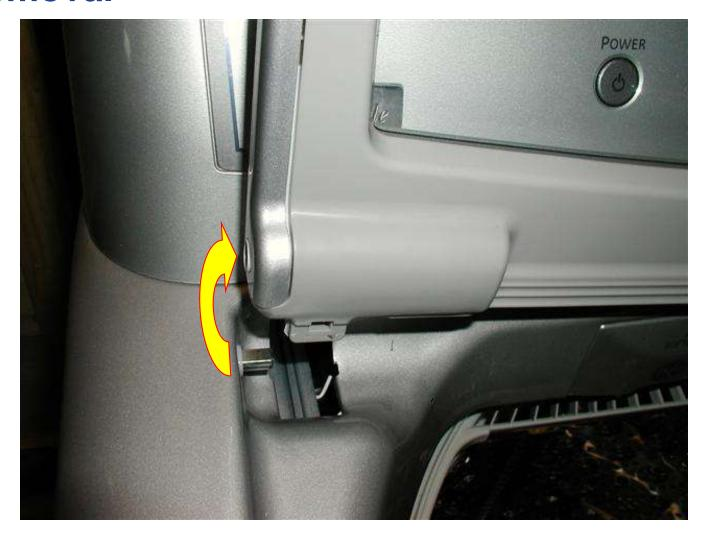
With hinge pin pulled completely to the left, lift left side of the lid upwards to clear pin....
