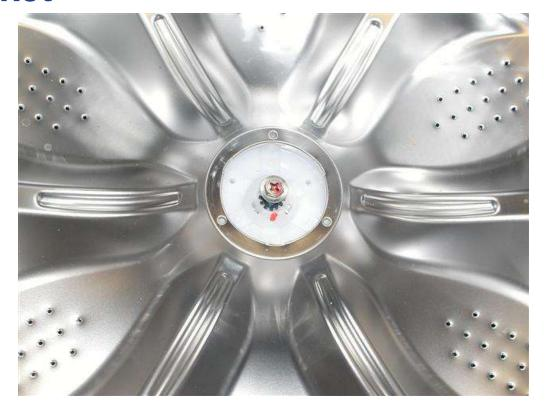
• Using a socket or Phillips-head screwdriver, remove the 10-mm hex-head screw that holds the infusor in place (turn screw counterclockwise to remove).
