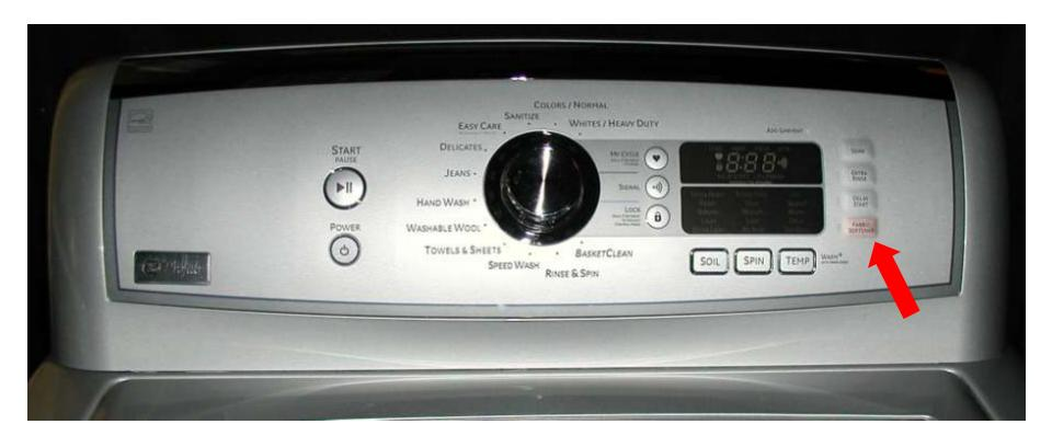
When the fabric softener pad is selected, the machine will provide a deep rinse instead of the spray rinse.
