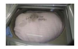
Worst case scenario in testing was with an overloaded tub with a pillow or pillows at the top of the load.
