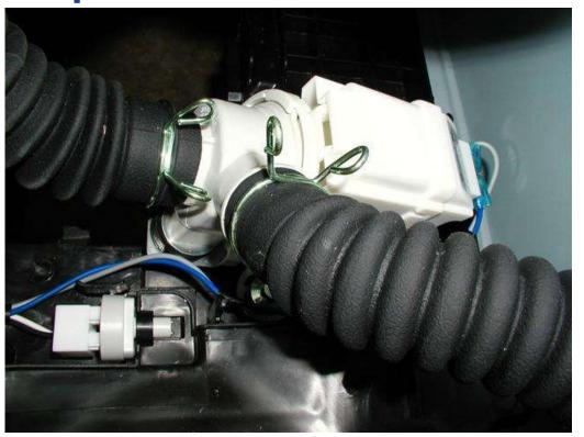
**Warning:** The drain pump bracket is not grounded. Unplug the unit before servicing to avoid electric shock.
