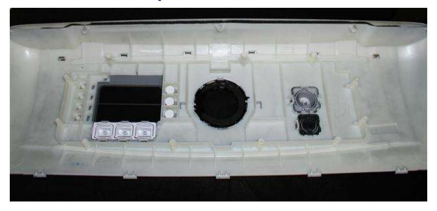
Selector buttons or pads are held to the control panel with tabs and are replaced as a complete assembly.
