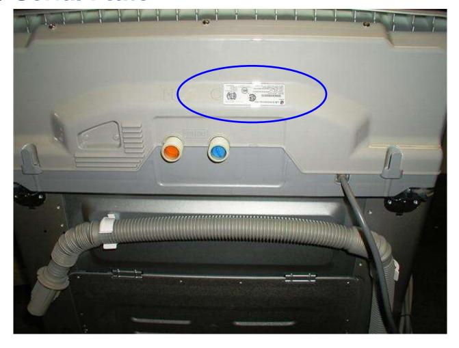
Model / Serial plate is located on the rear of the backsplash just above the water inlet connections.
