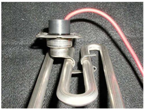
The reason for proper orientation of the thermostat is because the heater support is part of the thermostat body and must be positioned correctly for the heater to be installed.
