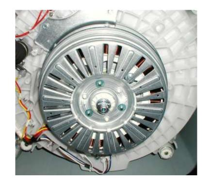
**Warning**: The rotor is not grounded & is moving when the motor is energized. Unplug the washer before servicing.
