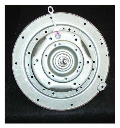
Remove the bearing housing assembly.
