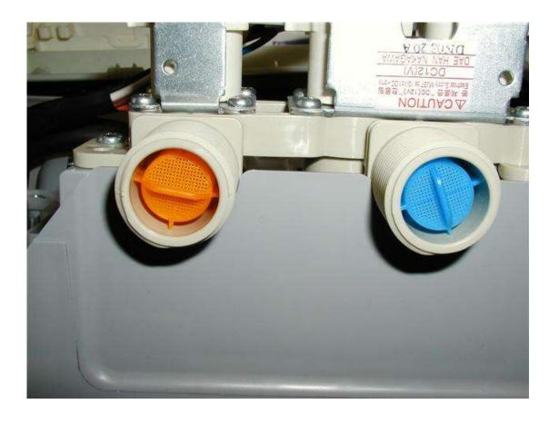
Hot and cold water inlet screens are used to prevent debris from entering the valve assembly.
