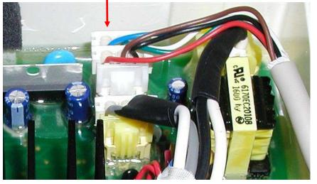
Lock assembly is secured to the underside of the washer top with two Phillips screws. The assembly includes the interconnect cable and plug. It connects to a six pin connector on the Main PCB at the plug shown above.
