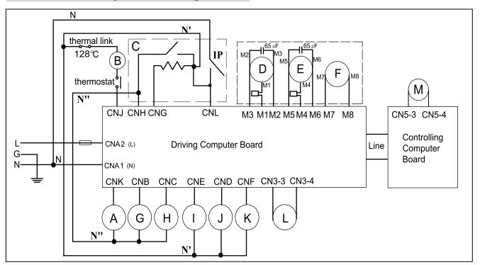
A:water inlet electromagnetic valve for hot water
