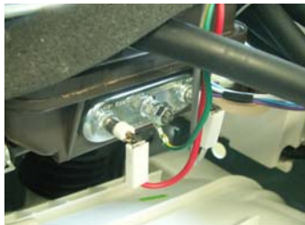
Steam generator heater
