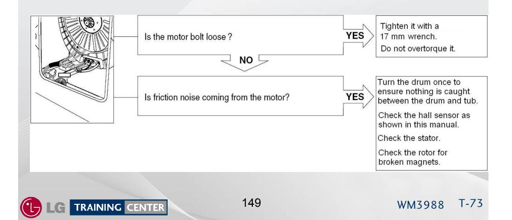
Several components of the machine can be tested before removing or exchanging them. Some test procedures can be completed without major disassembly other than to disconnect the component from its circuit; others may be tested from their connector on the control panel. Often, the only equipment required is a multimeter.
