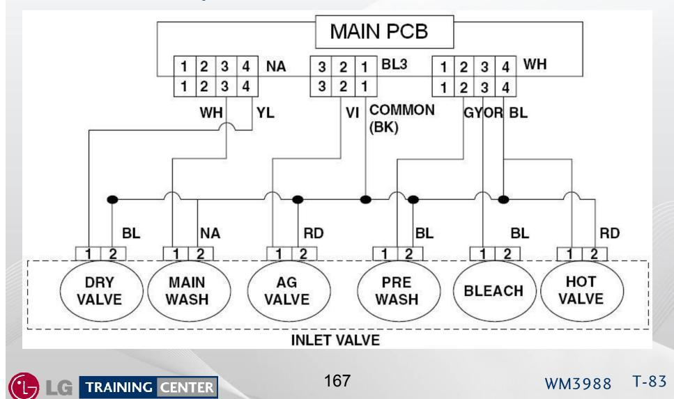
For all solenoids: With the solenoid connected and energized, the voltage should be 120 VAC. With the connector removed from the solenoid, the resistance should be 1.0  $\Omega \pm 20\%$ .
