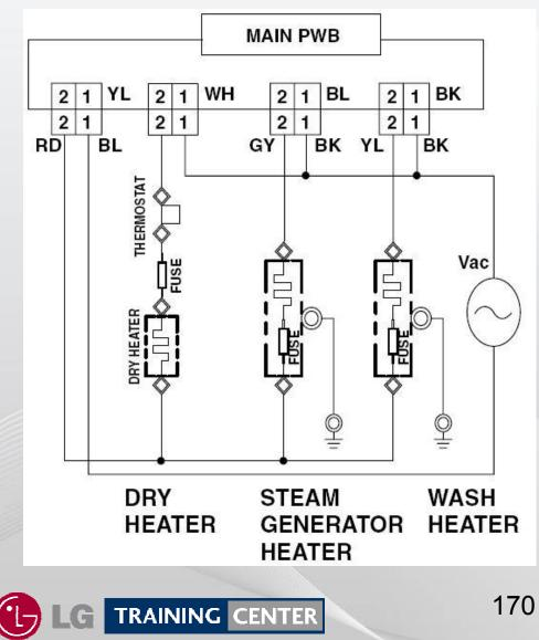
When using the connectors for test points, pay particular attention to connector and wire colors and numbers.
