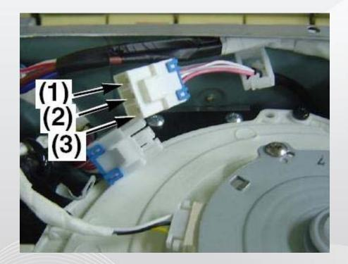
Test resistance (DA1) across terminals 1 and 2. 39.5 k $\Omega \pm 5\%$  at 86° (30° C) 26.1 k $\Omega \pm 5\%$  at 104° (30° C) 12.1 k $\Omega \pm 5\%$  at 140° (30° C) 8.5 k $\Omega \pm 5\%$  at 158° (30° C) 3.8 k $\Omega \pm 5\%$  at 203° (30° C) 2.8 k $\Omega \pm 5\%$  at 221° (30° C)
