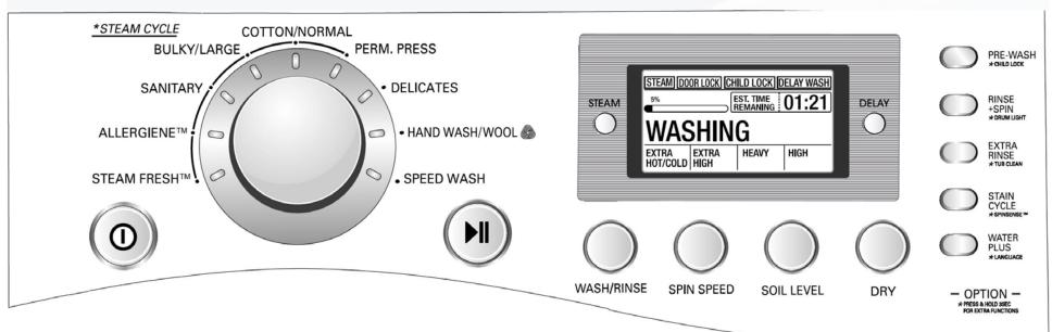
Power Button Cycle / Start Button Delay Wash Button Display Window Option Buttons
