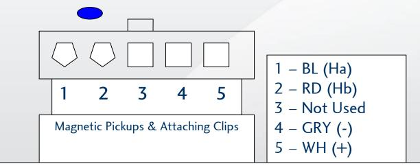
OHM CheckingVoltage Checking5 to 1 = 10 K  $\Omega$ 5 to 4 = 10 to 15 V<sub>dc</sub> Voltage Input5 to 2 = 10 K  $\Omega$ 4 to 1 = pulsing 10 V<sub>dc</sub> Signal Output4 to 2 = pulsing 10 V<sub>dc</sub> Signal OutputNote: Ohm values are approximate; if the ohm check determines either resistor open,<br/>the hall sensor has failed and must be replaced!!
