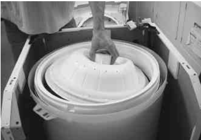
During reassembly orient the Tumbler facing up.
