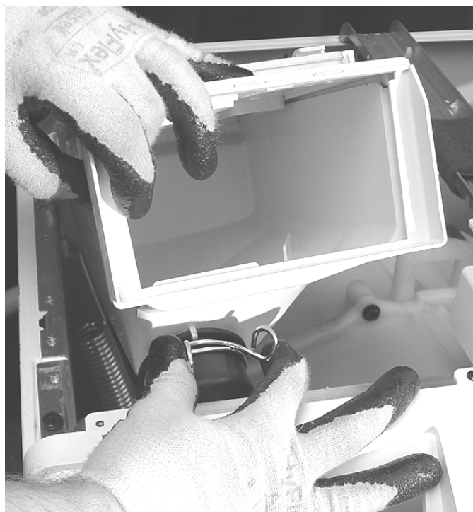
6. Remove fill hose clamp and hose.
