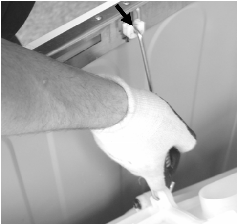
Long end of spring hooks on rail short end hooks to tub
