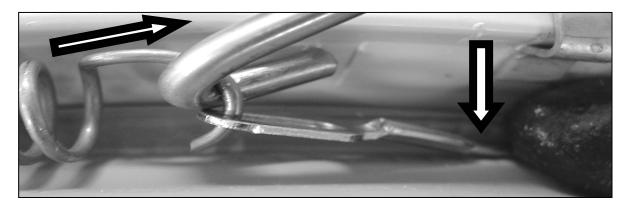
Hold the cable eyelet firmly down against the gasket. Hook the open end of the spring with the suspension tool and unhook from the eyelet
