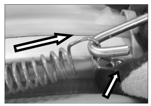
Position the open end of the spring face down. Use the suspension tool to expand the spring, and hook to the eyelet.
