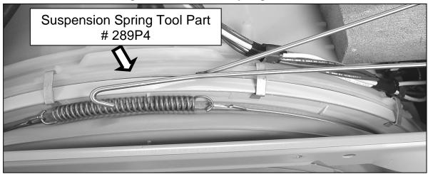
To remove or install boot spring and cable use suspension spring tool part # 289P4
