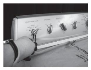
3. Remove three screws along the top of the Console and roll the Console forward.
