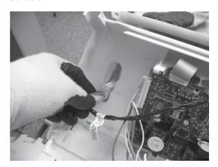
5. Disconnect all wiring harness connectors from the Circuit Board.
