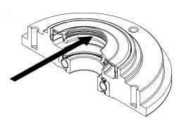
Apply grease to location indicated with arrow on Triple Lip Seal.
