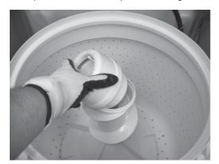
Remove screw located in the center of the Agitator/ Auger assembly.
