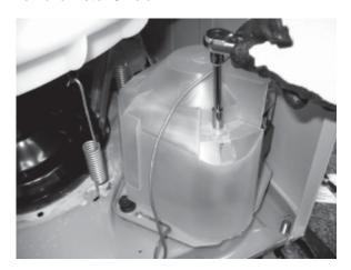
6. Remove Motor wire harness connector.
