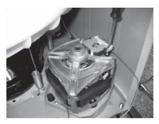
7. Remove three screws retaining Motor to Base.
