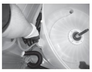
14. Remove Suspension Springs using the spring removal tool. Be careful not to let Tub and Transmission assembly tip over.
