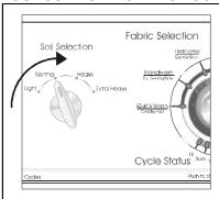
Press the Cycle Selection Knob to activate the test for the rotary switches. The test begins with the rotary switch imediately to the left of the Cycle Selection Knob. Rotate the switch in either direction. The LED's illuminate around the bottom of the Cycle Selection Knob for each switch position.
