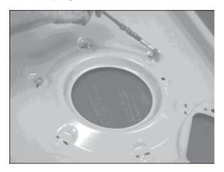
12. Clean the dome area of new Base with alcohol then apply corn starch.
