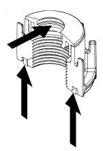
Apply grease to locations indicated with arrows on Seal Nut.
