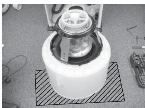
16. Mark location of Transmission Support with respect to the Outer Tub for ease of assembly.
