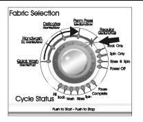
Rotate the Cycle Selector Knob clockwise past "Power Off" twice and stop at "Regular".
