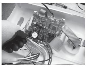
6. Depress the PCB locking tab and remove Circuit Board.
