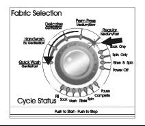
Rotate the Cycle Selector Knob counterclockwise one revolution back to "*Regular*" and *press* knob.
