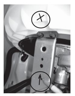
17. Remove screws retaining Outer Tub to Transmission Support.
