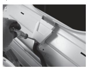
6. Remove hose clamp and Flume/Diverter Hose.
