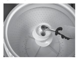
7. Remove Agitator Auger from Agitator Base.
