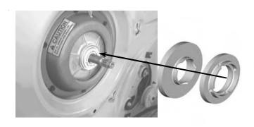
2. Apply a thin layer of **grease** between the contacting surfaces of the Lower Cam and the Drive Pulley.
