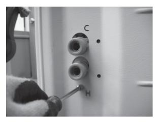
4. Lift Water Valve to align with cutout in back cabinet.
