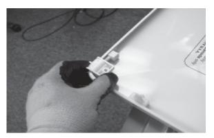
5. Remove Lid Switch Striker by removing screw from the Lid side.
