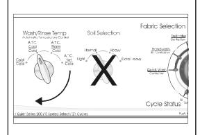
Press the Cycle Selection Knob. The test continues with the switch immediately to the left of the previous switch tested. Repeat rotating the switch and monitoring the LED's around the bottom of the Cycle Selection Knob. Continue pressing the Cycle Selection Knob for each switch tested right to left untill all rotary switches are tested.
