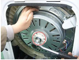
Slide a Philips screw driver into a hole in the rotor and through a stator winding. This will keep the rotor from spinning the drum when loosening the nut. Using a 19mm wrench or socked, remove the retaining nut and washer
