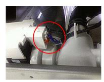
Remove the connector and read the resistance at the terminals on the Drain Pump: Should be 14  $\Omega$
