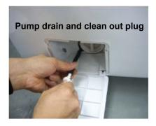
Remove the front access panel to the pump clean out filter and drain the excess water.
