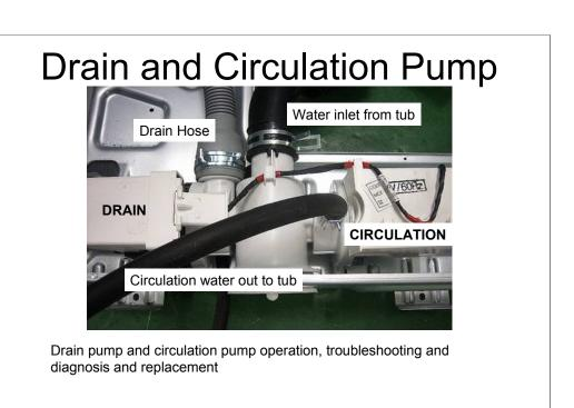
This module will explain the drain pump operation and some troubleshooting tips as well as the procedure for replacement.
