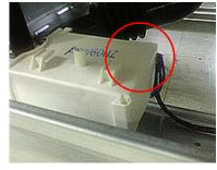
Remove the connector read the resistance at the terminals on the Circulation Pump: Should be 28  $\Omega$
