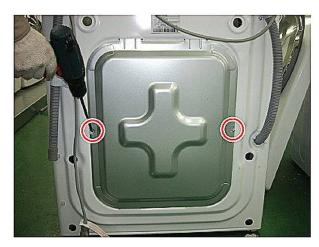
Remove the rear access panel to uncover the drum motor
