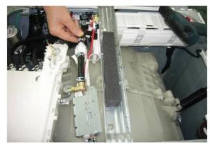
With the screws removed, disconnect the wiring harness and water lines to the steam unit and remove. Reverse the procedure to install the new steam unit.
