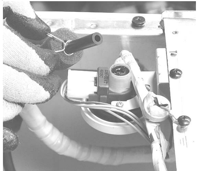
17. Remove ground wire.
