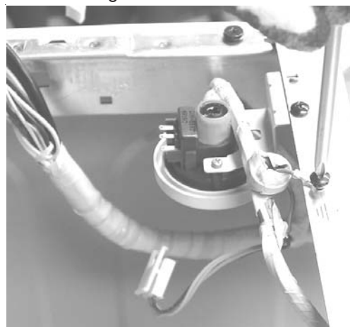
17. Remove ground wire.
