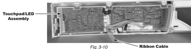
The Touch Pad/LED Assembly, (Fig. 3-10), is removed as a single assembly and is connected to
