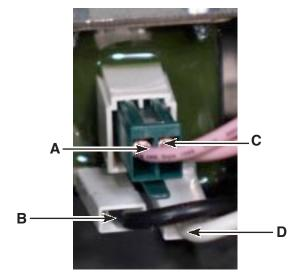
A to B = 0 ohms C to D = 0 ohms
