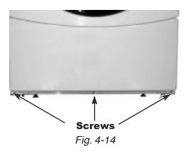
Remove the two screws securing the bottom of the front panel to the washer, and the two screws securing the top of the front panel to the washer. The front panel can now be removed from the washer. (Fig. 4-15)
