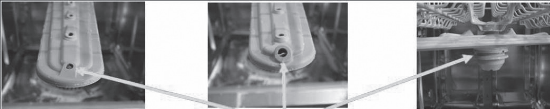
Blocked Spray holes and stalled spray arm rotation
