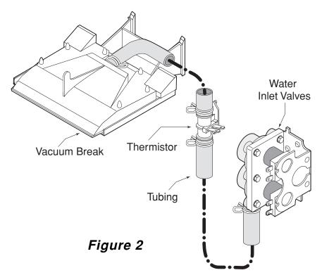
The ATC board uses the input from the thermistor to cycle the hot and cold water solenoids on the water inlet valves to achieve the desired water temperature setting. A triac, located on the control board, cycles the hot and cold water solenoids through the temperature relay and the water temperature switch (see Figure 3).
