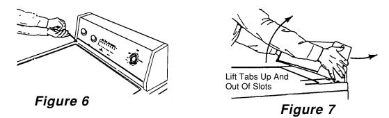
3. Carefully rotate the console so that the back faces you. **NOTE: Do not lay the console** against a wall without a protective cover or you may scratch it.
